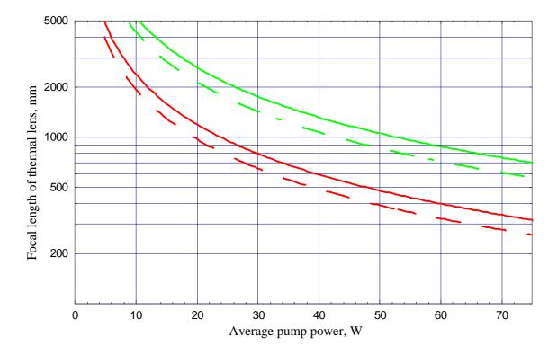
Fig. 5.4. Calculated focal lengths of thermal lens for Brewster-cut crystal [Wagner, 2009]. Pump beam diameter 2.1 mm. Values in tangential plane marked red, in sagittal – green. With a solid curve are plotted results for simulation of the laser operation at 820 nm, with a dashed curve – at 935 nm.
