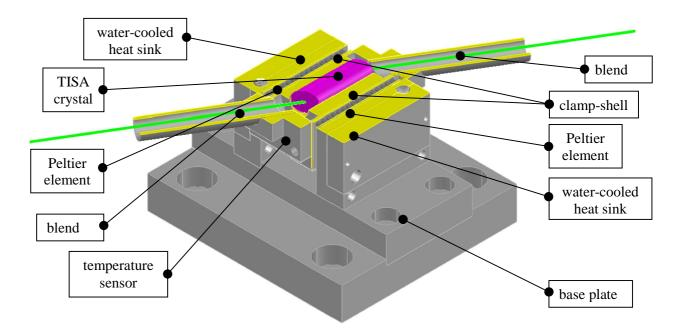
Fig.5.3 Scheme of the clamp-shelled TISA crystal mounted into the heat sink (courtesy of Gerd Wagner, IPM, Uni Hohenheim).
