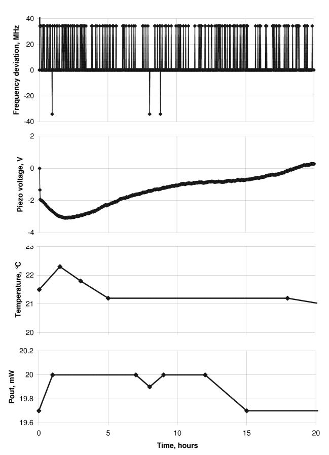
Fig.4.7 Long-term test of the IS on the base of the Toptica DL100 system at 935 nm. From top: IS frequency deviation, value of correction signal, temperature, output power.
