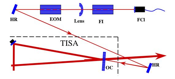
Fig.4.11 Coupling of the fiber output of the IS into the TISA cavity. Here FCI - fiber collimator, FI - Faraday isolator, Lens – negative lens of the beam shaper, EOM – electro-optical phase modulator, OC – output coupler, HR – high-reflective mirrors, CCD – CCD-camera.
