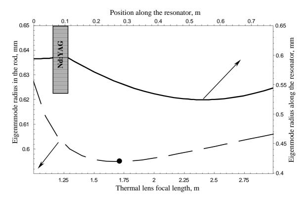
Fig.3.4 Calculated stability zone of the MO, the eigenmode size in the rod as a function of the thermal lens focal length (dashed curve), and the eigenmode size along the resonator, starting at the back HR mirror (solid curve). Current thermal lens focal length value is marked with a circle.
