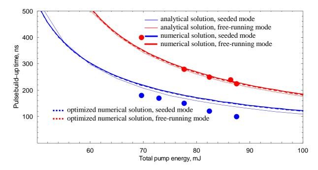
Fig.5.16 Pulse build-up time of the TISA laser at 935 nm vs. absorbed pump energy, measured for seeded (blue dots) and not seeded (red dots) operation. Result of the modeling is drawn with thin, thick and dashed curve for the analytical, numerical, optimized numerical solution, respectively. Conditions of the experiment and assumption of the calculations were the same as for the slope efficiency (see Fig. 5.14).
