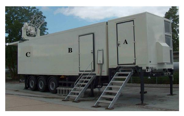
Fig.6.2 Photo of the mobile platform for the water-vapor DIAL. A – energy module, B – laboratory module and C – telescope compartment.
