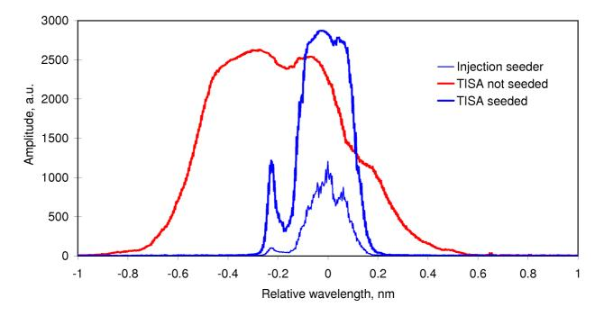
Fig.5.17 Coarse spectrum of the IS and the TISA laser, seeded and not seeded, obtained with the grating spectrometer SPEX 1302 (resolution  $\approx 0.2$  nm @ 930 nm). The subpeakes are due to misalignment of the coupled laser beam.
