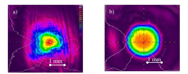
Fig.5.33 Cross-section of the pump beam a) and TISA beam at 825 nm b) with the pump laser in the configuration Pump-2.
