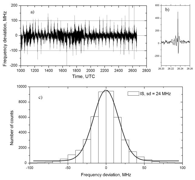
Fig.4.10 Frequency deviation of the IS during DIAL measurements on 01-02 Aug 2007: long-term trend (a), detailed picture of a mode hop (b) and statistical distribution (c). Here sd – standard deviation
