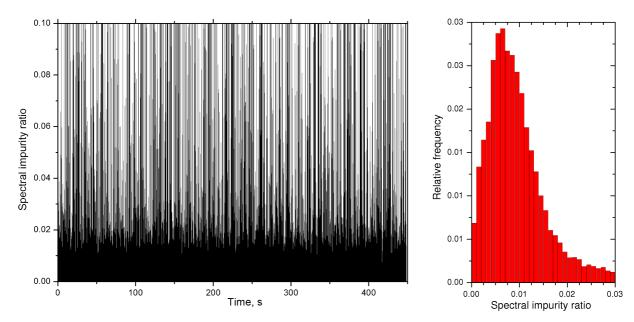
Fig.5.40 Spectral impurity measurement of the TISA transmitter with a DIAL-system in coaxial configuration. Here is presented shot-to-shot 450 s trend of the spectral impurity ratio  $I_{on}/I_{off}$  (left) and the correspondent statistics (right). Assuming all the negative data having a noise nature, they were removed from the final statistics.
