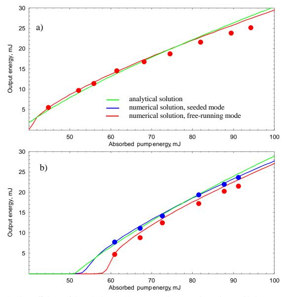
Fig.5.29 Slope efficiency of the TISA laser at 825 nm, operating near gain maximum with the pump source in configuration Pump-1, for a broad-band operation, without BF (a) and for narrow-band operation, with BF (b). Experimental results are marked with dots, numerical solution of the pulse evolution model are drawn with curves of red and blue color for free-running and seeded mode, respectively. With a green curve the analytical solution of this model is drawn.
