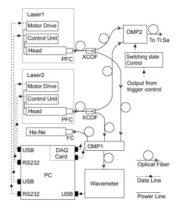
Fig.4.9 Principle scheme of the IS developed at DLR. Here FC – Fiber coupler, PFC – Precision Fiber Coupler, XCOF – Cross Coupled Optical Fiber, OMP – Optical Multiplexer, HeNe – helium-neon laser. Courtesy of DLR Oberpfaffenhofen.
