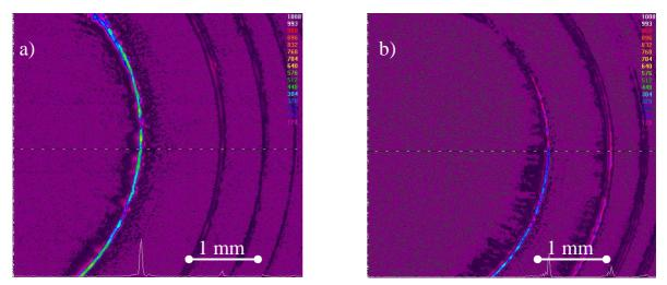
Fig.5.37 Fringe patterns of the laser emission build in a confocal FPI and recorded with a CCD-camera. Here are the measurements of the seeded TISA laser (a) and the single-mode cw IS (b) at 820 nm. The shots were shifted rerding the center of the fringes to capture simulteneously at least three rings for an accurate definition of the departure of the mirrors and magnification of the optics.
