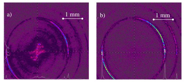
Fig.5.18 Fringe pattern formed in the confocal FPI and recorded with a CCD-camera for a) partially seeded TISA and b) injection-locked TISA at 935 nm.
