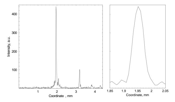
Fig.5.38 Intensity distribution in the fringe pattern of the injection-locked TISA laser at 820 nm along the horizontal main axis of the fringes (left); corresponds the horizontal dashed line on the Fig. 5.38 (a). Scaled cross-section of the first-order ring is imaged on the right, cell width of the CCD-array is 8.6  $\mu$ m.
