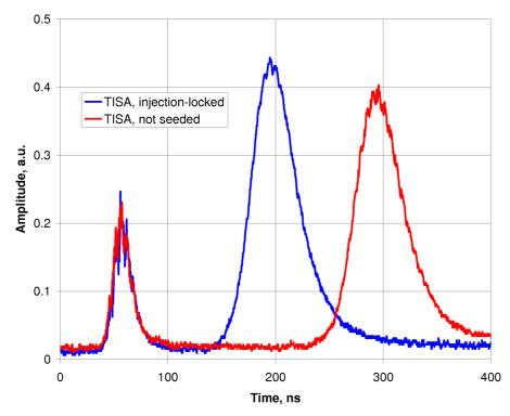
Fig.5.35 Temporal profile of the pump pulse at 523 nm (the first of three) and TISA pulse at 825 nm, seeded (blue) and free-running (red) in configuration Pump-1. A small mode beating in the seeding mode is notable.
