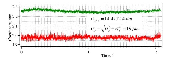
Fig.5.34 Trend of the beam position of the TISA laser at 825 nm in horizontal (green) and vertical (red) planes; the beam was monitored at the distance of 1.5 m from the OC.
