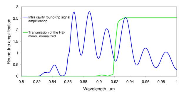
Fig.5.10 Calculated spectrum of the small-signal intra-cavity round-trip amplification in the TISA laser at 935 nm. Cavity round-trip amplification without HE-mirror (blue), reflectivity of the HE-mirror, normalized to the peak of round-trip amplification (green).
