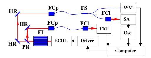
Fig.4.5 Set-up of the IS. Here ECDL – external-cavity diode laser, FI – Faraday isolator, PR – partially reflecting mirror, HR – high-reflecting mirror, FCp – fiber coupler, FS – fiber splitter, FCl – fiber collimator, PM – power meter, WM – wavemeter, SA – spectrum analyzer, Osc – oscilloscope.
