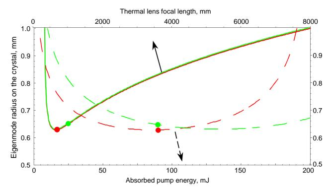
Fig.5.12 Calculated radius of the  $\text{TEM}_{00}$  in the crystal rod with respect to the thermal lens focal length (solid curves) and absorbed pump energy (dashed curves) in tangential (red) and sagittal (green) planes. The radii values corresponding the maximum pump power are marked with disks. The correlation between the thermal lens values and the pump power was established regarding the experiment described in Subsection 5.2.4.
