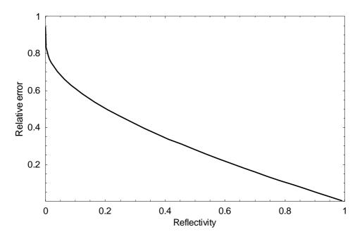
Fig.A.1 Estimated relative error of the point-resonator model vs. reflectivity of the OC.
