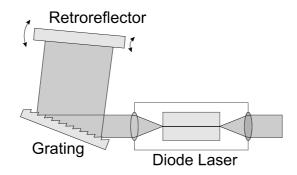
Fig.4.8 Principle design of an ECDL in Littman/Metcalf configuration (after www.sacher-laser.com).
