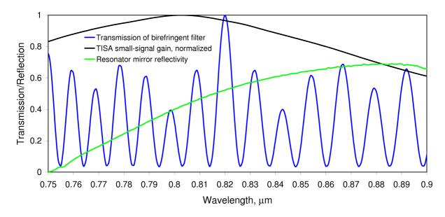
Fig.5.24 Calculated spectral properties of the intra-cavity elements of the TISA set-up at 820 nm: TISA small-signal gain, normalized (black); calculated transmission spectrum of the 4-plate BF, optimized for 820 nm (blue); round-trip reflectivity of the three HR and OC of the z-shape ring cavity (green).
