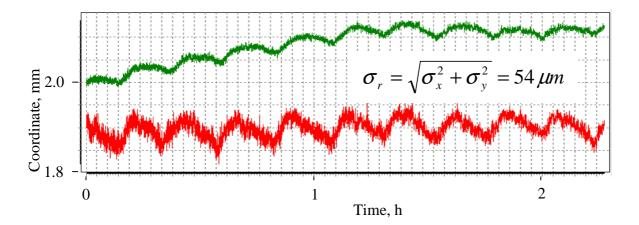
Fig.6.4 Trend of the beam pointing of the TISA laser recorded in the DIAL trailer for horizontal (red) and vertical (green) components. Recorded with a CCD-camera 2.5 m away from the OC of the TISA.
