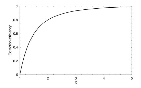
Fig.A.2 Extraction efficiency of the stored energy regarding ratio  $X = \frac{g_0}{\beta_{\Sigma}}$ , representing an exceeding of the small-signal gain over the total losses (see also [Siegman, 1986, p.1015]).
