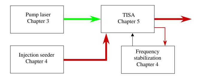
Fig.2.2 Principal scheme of the transmitter for the water-vapor DIAL.
