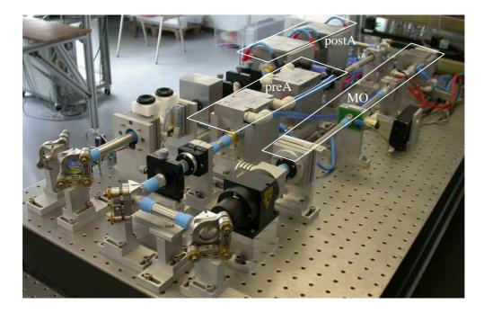
Fig.3.2. Layout of the pump laser corresponding the scheme 3.1, used without IS for this work. The size of the breadboard is 120x60 cm.
