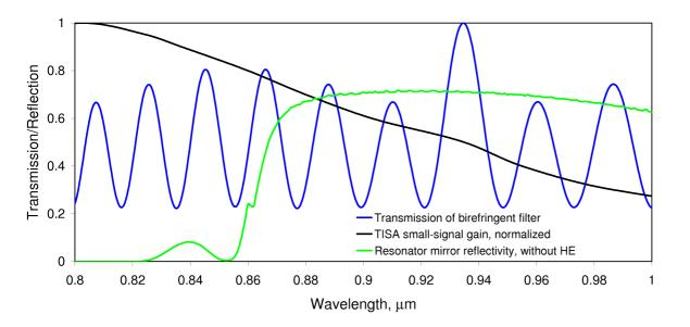
Fig.5.9 Calculated spectral efficiency of the intra-cavity elements of the TISA set-up at 935 nm: TISA small-signal gain, normalized (black); calculated transmission spectrum of the 3-plate BF, optimized for 935 nm (blue); round-trip reflectivity of the three HR and 70% OC of the Z-shape ring cavity (green).
