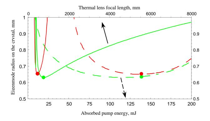
Fig.5.27 Calculated radius of the  $TEM_{00}$  in the crystal rod with respect to the thermal lens focal length (solid curves) and the absorbed pump energy (dashed curves) in tangential (red) and sagittal (green) planes. The radii values corresponding the maximum pump power are marked with disks.
