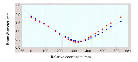
Fig.5.31  $M^2$ -measurement of the TISA beam at 825 nm with the pump laser in configuration Pump-1, red points correspond to the beam cross-section in tangential plane, blue – in sagittal.
