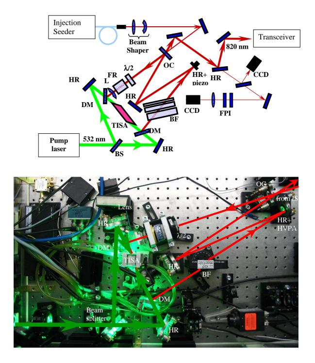
Fig.6.3 Scheme of the set-up of the TISA laser at 820 nm and photo of the TISA cavity during COPS. Here beam splitter (BS), high-reflective mirrors (HR), dichroic mirrors (DM), output coupler (OC), Faraday rotator (FR), birefringent filter (BF), Fabry-Perot interferometer (FPI), halfwave plate ( $\lambda$ /2), HR mirror, glued on a piezo actuator (HR+HVPA).
