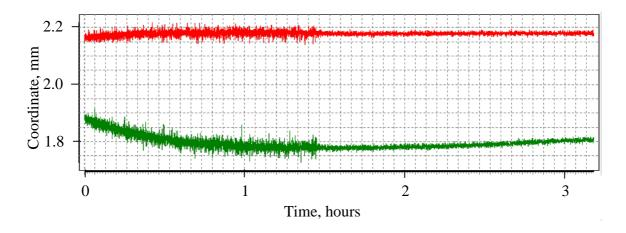
Fig.3.10 Spatial stability of the pump beam (after MO, IR); red – horizontal plane, green – vertical. Higher fluctuation first 1½ hour is caused by implementing of a single-shot acquisition, whereas later a 4-shot averaging was applied.
