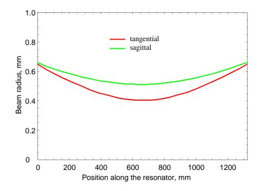
Fig.5.11 Calculated radius of the eigenmode along the resonator in tangential (red) and sagittal (green) plane, respectively. The 0-position corresponds the first principle plane of the TISA.
