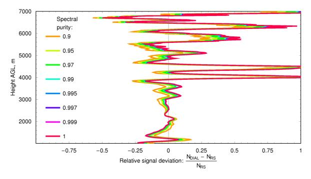
Fig.5.43 Relative deviation between DIAL and radiosonde signals for measurement on 1<sup>st</sup> Aug 2007, 1100 UTC. A spectral-impurity correction was applied to the DIAL profile, averaged around the launch time of the RS. Different curves on the plot corresponds different levels of the estimated spectral purity of the DIAL emission, from 90% to 100%. The one with the smallest bias indicates the expected value of the spectral purity.
