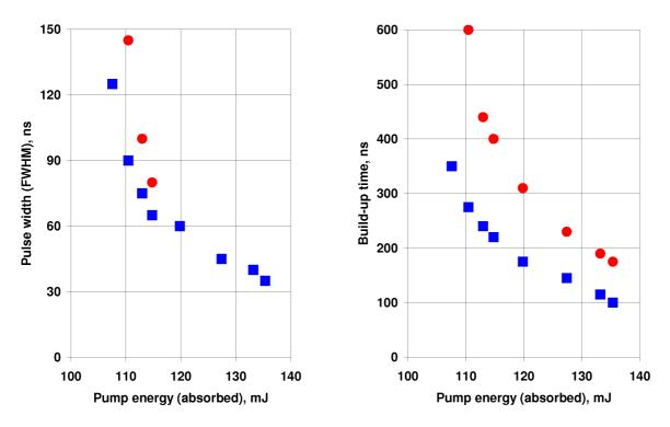
Fig.5.36 Pulse width (left) and pulse build-up time (right) of the TISA laser at 825 nm vs. absorbed pump energy. Results of the TISA with seeded emission marked blue, free-running – red.
