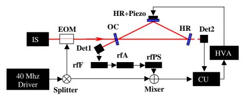
Fig.4.2 PDH stabilization scheme adopted for a ring cavity. Here EOM – electro-optical phase modulator, HR – high-reflecting mirror, OC – output coupler, Det1, Det2 – biased photodetectors, rfF – rf-filter, rfA – rf-amplifier, rfPS – rf-phase shifter, CU – control unit, HVA – high-voltage amplifier.
