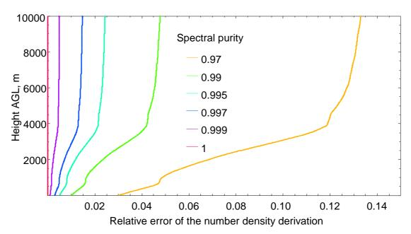
Fig.5.42 Relative value of the spectral-impurity induced error for derivation of the water-vapor information from a DIAL-measured profile on variuos heights. Atmospheric conditions are simulated regarding the radiosonde measurement on 01 Aug 2007, 1057 UTC, Hornisgrinde.
