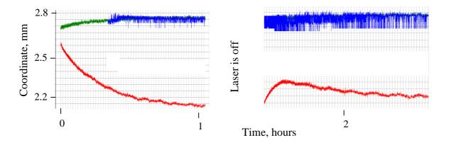
Fig.3.11 Spatial stability of the pump beam (on the TISA-crystal, 532 nm); red – horizontal plane, green(blue) - vertical plane. The overlapping blue trend is a momentary position of the beam peak in vertical direction.
