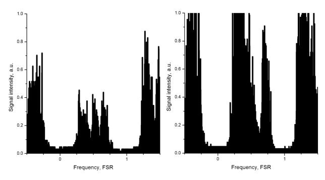
Fig.5.20 Intensity of the unseeded TISA emission while scanning the IS frequency over the range of several FSRs of the slave cavity. Measurements made with IS power of 16 mW and TISA output of 1.8 W (left) and 2.8 W (right). The multiple subpeaks are due to a frequency beating of the acquisition system of the oscilloscope and the pump laser repetition rate.
