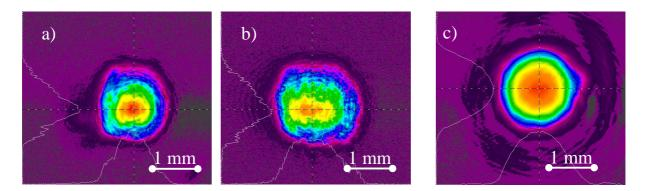
Fig.5.30 Cross-section of the pump beam and TISA beam at 825 nm with the pump laser in the cofiguration Pump-1. Pump beam for the experiment without BF (a) and with BF (b), TISA beam(c).
