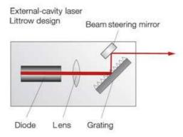
Fig.4.4 Principle design of an ECDL in the Littrow configuration (after www.toptica.com)
