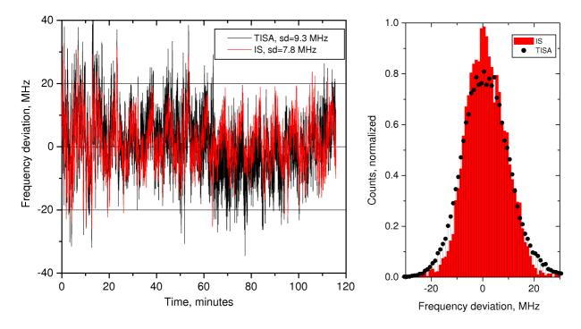
Fig.5.39.Measured frequency deviation of the injection seeder (red) and injection-locked TISA laser (black) within a 2-hour trend (left) and its statistics (right).
