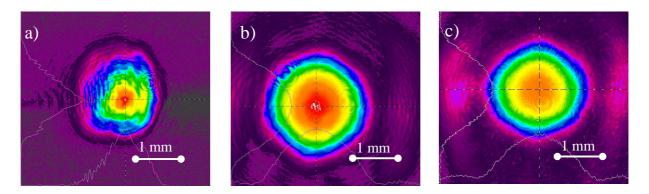
Fig.5.15 Cross-sections of the pump beam (a) and the outcoupled cavity mode of the injection-seeded TISA at 935 nm: 68 mJ pump, 11 mJ output (b) and 75 mJ pump, 15 mJ output (c).
