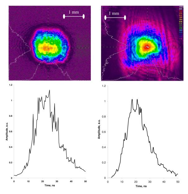
Fig.3.7 Pump energy distribution on the TISA-crystal (up) and temporal profile of the not seeded pump pulse (down) in Pump-1 (left) and Pump-2 (right). Wavelength 532 nm.
