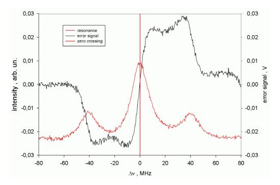
Fig.4.3 Signals in a PDH stabilization circuit: relative IS frequency with sidebands (red curve) and error signal (black curve). Resonance position is marked with a red line (regarding [Wulfmeyer et al., 2000a]).
