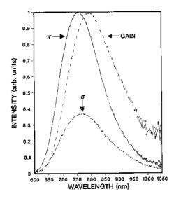
Fig.5.1 TISA polarized fluorescence spectra and calculated gain line shape [Moulton, 1986].
