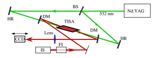
Fig.5.5 Scheme of the set-up for a measurement of the thermal lens. Here BS – beam splitter, HR – high-reflective mirror, DM – dichroic mirror, IS – injection seeder, FI – Faraday isolator, CCD – CCD camera.
