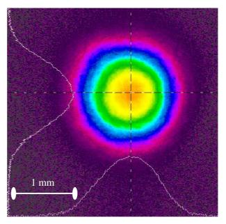
Fig.3.5  $M^2$ -measurment of the MO beam in the horizontal (x, red) and vertical (y, blue) planes.
