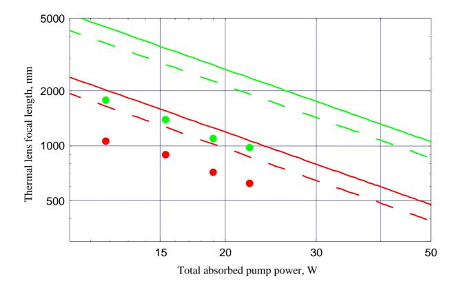
Fig.5.6 Experimental and theoretical values of the thermal lens focal length in a Brewster-cut crystal rod vs. absorbed pump power. For the pump laser in configuration Pump-1, measured values marked with points, theoretically derived values [Wagner, 2009] are drawn with curves. Values in tangential plane marked red, in sagittal – green. With a solid curve the results for simulation of the laser operation at 820 nm are plotted, with a dashed curve – at 935 nm. Beam diameter 2.1 mm.
