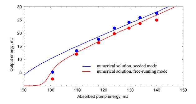
Fig.5.32 Slope efficiency of the TISA laser at 825 nm with the pump laser in configuration Pump-2 in seeded (blue) and free-running (red) modes. Experimental results marked with circles, results of simulation with solid curves of the corresponding colors.
