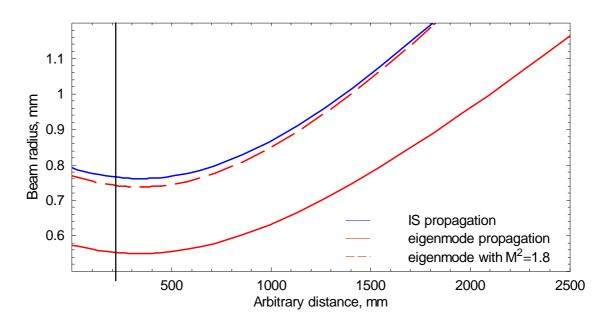
Fig.4.12 Fitting of the beam propagation of the IS (blue) to the eigenmode of the cavity (solid red). Dashed red line corresponds the intra-cavity mode with  $M^2 = 1.8$ . Waist position of the intra-cavity eigenmode is marked with a black line.
