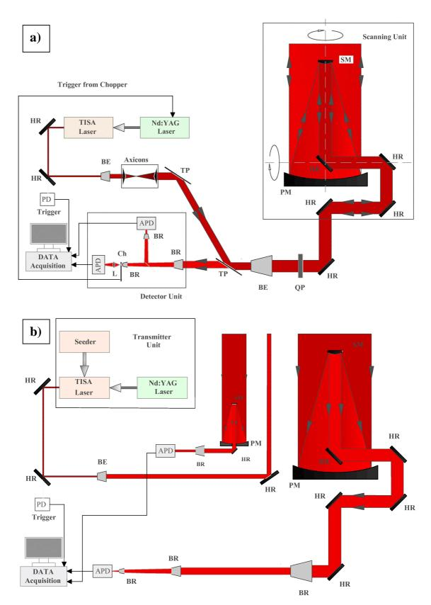
Fig.6.1 Principle scheme of the water-vapor DIAL in coaxial (a) and bi-axial (b) configurations (courtesy of Dr. Riede, IPM). Here: BE – beam expander, TP – thin-film polarizer, QP – quarter-wave plate, HR – high-reflection mirror, PM and SM – primary and secondary mirrors of the telescope, BR – beam reducer, Ch – fast chopper, L – lens, PD – silicon photodetector, APD – avalanche photodetector.
