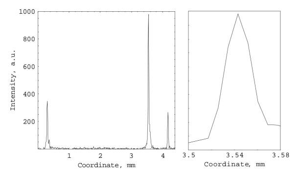
Fig.5.19 Intensity distribution in the fringe pattern of the injection-locked TISA along the horizontal main axis of the fringes (left); corresponds the horizontal dashed line on the Fig. 5.18 (b). Scaled cross-section of the first-order ring is imaged on the right, cell width of the CCD-array is 8.6 µm.
