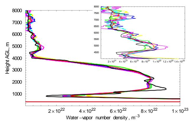
Fig.5.41 Water-vapor number density profiles, obtained with the DIAL (color curves) and radiosonde (black curve) from 1 August 2007 1020-1135 UTC, Hornisgrinde. DIAL profiles are averaged over 15 minutes and have a 600-m window gliding. Radiosonde data was smoothed with a 150-m gliding window.
