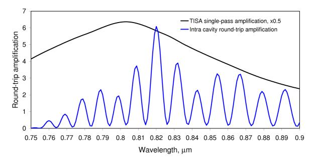
Fig.5.25 Calculated spectrum of the small-signal intra-cavity round-trip amplification in the TISA laser at 820 nm. TISA small-signal single-pass gain (black) scaled 0.5, cavity round-trip amplification (blue).
