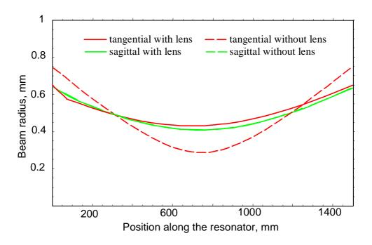
Fig.5.26 Calculated radius of the eigenmode along the resonator of the TISA set-up at 820 nm in the tangential (red) and sagittal (green) plane. Beam propagation along the cavity with the lens is marked with a solid line, without the lens with dashed line.
