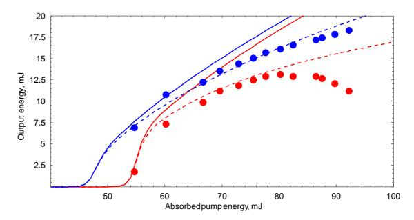
Fig.5.14 Slope efficiency of the TISA laser at 935 nm. The results for the free-running mode marked red, for the seeded – blue. Experimental data marked with dots, numerical solution – with solid lines, numerical solution with intensity-dependent losses – with dashed lines.
