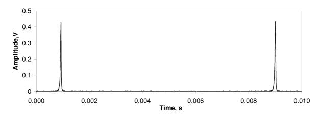
Fig.4.6 Spectrum of the IS at 935 nm, recorded with the spectrum analyzer. Having FSR = 7.5 GHz and finesse > 250, the SA defines the single-mode operation of the IS with an ucertainty < 30 MHz, limited by the resolution of the instrument.
