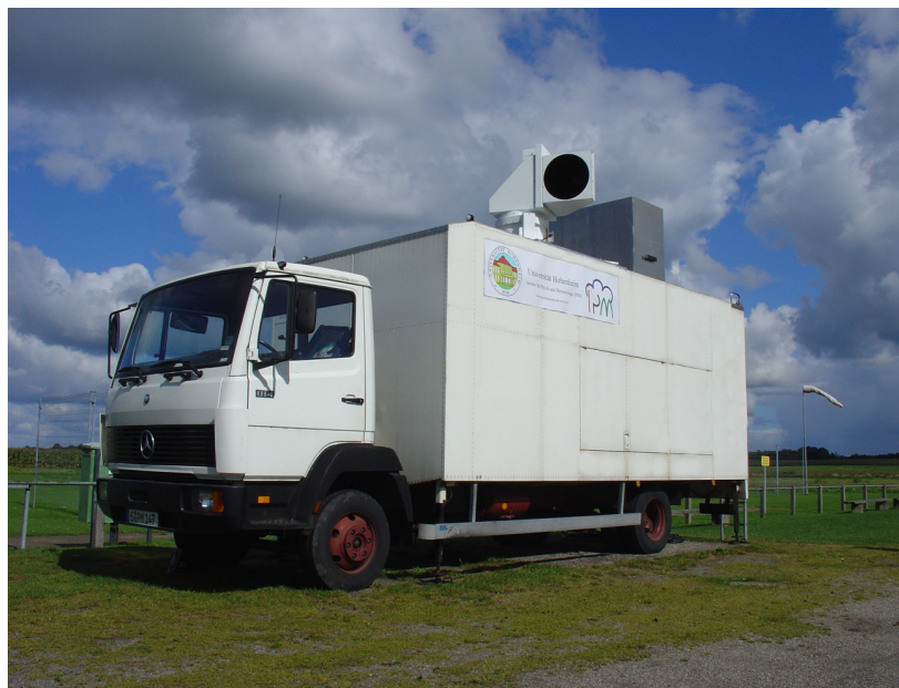
Figure 3.7: Mobile platform including the scanner of the UHOH scanning lidar in operation during a field campaign in 2005.
