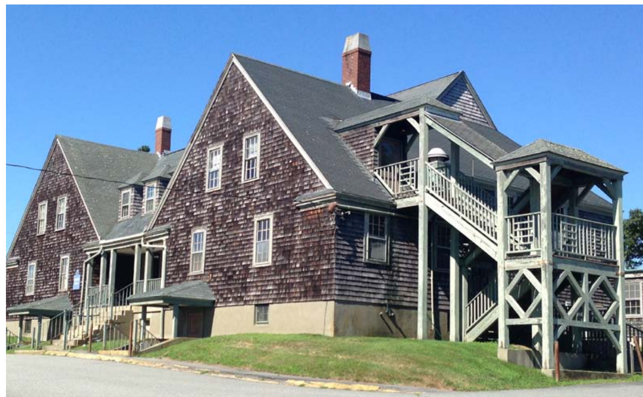
The parish house is classified as Shingle style architecture because of its exterior wooden shingles, gabled roofs, multi-light windows and porch.
