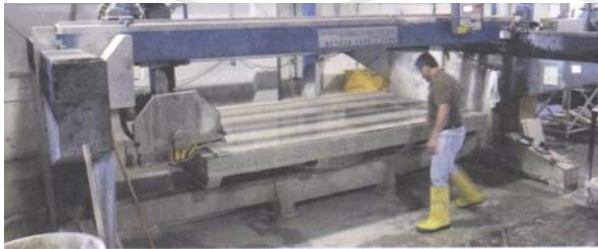
CNC stone-cutting gantry saw at Pacific Westline, Inc.
