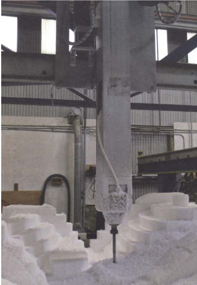
CNC machine milling formwork for the bloom house_Greg Lynn Form
