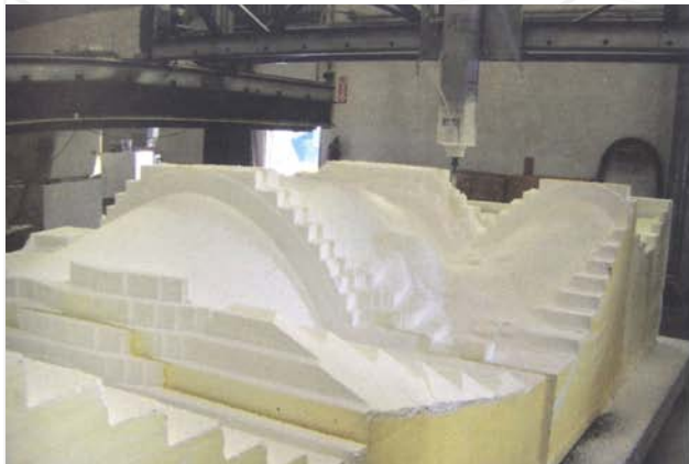
CNC formwork-workers molding fiberglass onto formwork for bloom house_Greg Lynn Form
