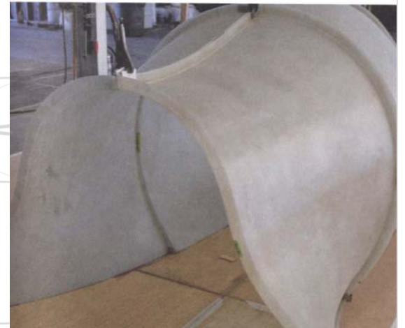
Finished fiberglass panels for bloom house_Greg Lynn Form
