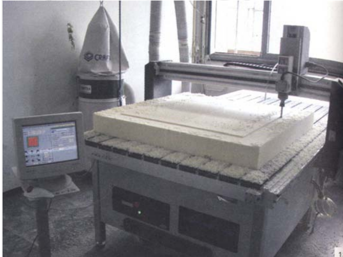
CNC mill making formwork for Intricate Surfaces exhibition display case_Greg Lynn Form
