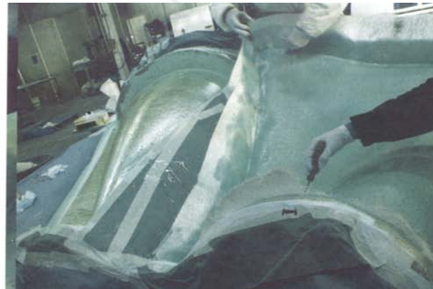
CNC formwork-workers molding fiberglass onto formwork for bloom house_Greg Lynn Form
