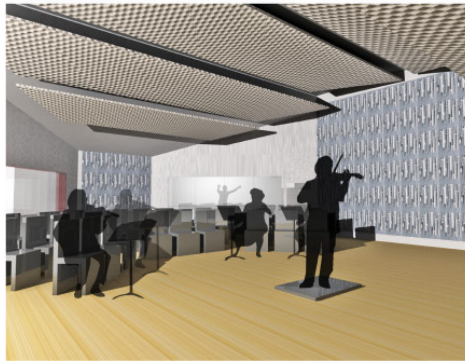
ACOUSTIC ANALYSIS IMAGES The strategy of urban blocks and raised bars are taken into account for an acoustic panel subjected to sound changes and energy profiles. The size and density work to create clarity.
