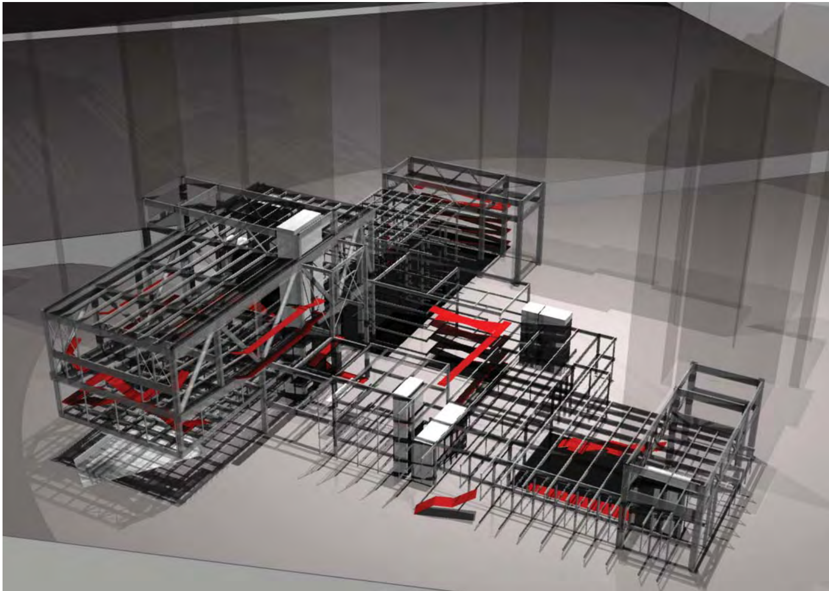
Vertical Circulation and Mechanical Cores
