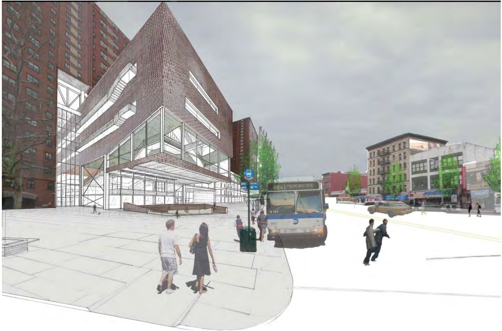
The cantilever envelope is shown here with a perforated metal. This was part of an experiment to create a semi-transparent wall.
