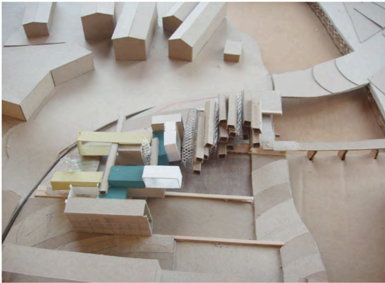
These explore the reverse order of the streetfront courtyard spaces. Here, the grow spaces and laboratories are put in the back, facing the river, and the classrooms are brought to the urban condition.
