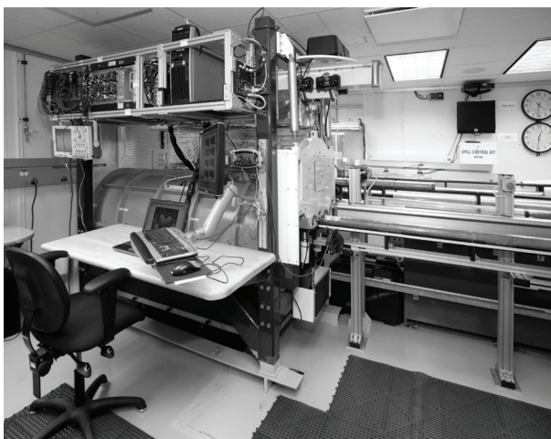
Figure 1. The natural gamma radiation (NGR) system on the JOIDES Resolution (from Vasiliev et al., 2011).
