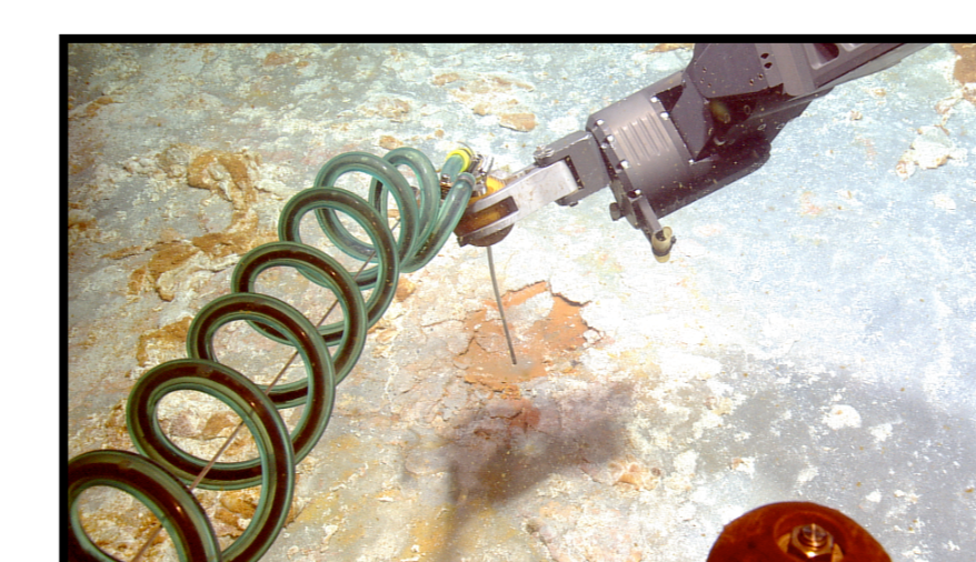
Fig. 8 Taking the temperature of the white bacteria mats. Temperature reading: 58°C, ambient 16°C
