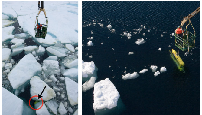
Fig. 2. The size of open leads and density of the ice during AUV recovery varied greatly from dive to dive. Opening a pond sometimes also required moving the ship, temporarily precluding AUV communications. The AUV is barely visible in the left image.
