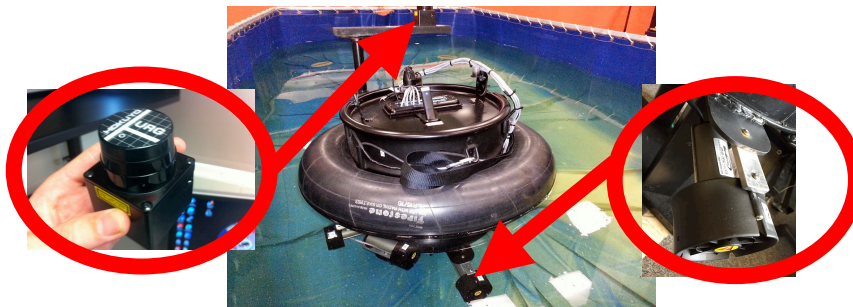
Figure 1. Robust Dynamic Positioning Vessel (Middle), LIDAR Sensor (Left), and SeaBotix Thruster (Right)
