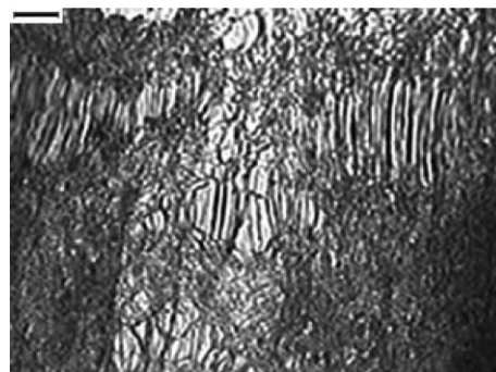
Fig. 5 Optical microscopy image showing long range alignment of silica. Scale bar = 50 \mu\text{m} .
