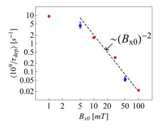
FIG. 1. Comparison of spin flip loss rate calculated in Ref. [21] for the Los Alamos UCN $\tau$  trap [20] using a 1D field model (blue squares) with the present 3D calculation for the smooth field given in Eq. (5) of [20] (red circles). In the range  $B_{x0} \gtrsim 5$  mT the data are represented reasonably well by the power law  $\langle 1/\tau_{dep} \rangle \sim B_{x0}^{-2}$ , as shown by the dashed line.
