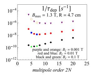
FIG. 2. Mean spin flip rates calculated from Eq. (20) for a cylindrical multipole trap vs order 2N. The purple, red, and black points (down triangles, closed circles, and diamond symbols) represent integer N; the intervening orange, blue, and green points (open circles, squares, and up triangles) are for half-integral N.
