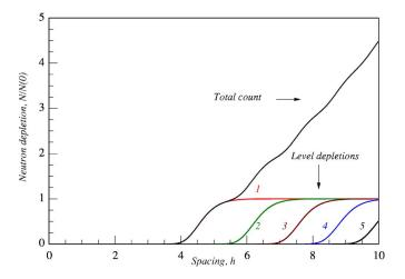
FIG. 11. (Color online) The neutron count N/N(0), Eq. (73), and individual depletions of the lowest energy levels, Eq. (74), as a function of the spacing between the walls *h* at  $\chi$ =0.15, *r*=0.015,  $\eta$ =30*r*. All higher levels are already depleted.
