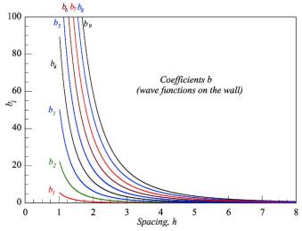
FIG. 7. (Color online) The coefficients  $b_j(h)$ , Eq. (71), which determine the square of the wave function on the surface of the scatterer,  $B_i^2$ .
