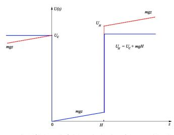
FIG. 1. (Color online) Schematic drawing of the potential well in vertical direction z. Dashed lines, the "real" potential; solid lines, the potential used in the paper. Since  $mgH/U_c \sim 10^{-5}$  and we are particularly interested in the lowest energy levels, the corrections are negligible (with an accurately scaled potential, the difference between the dashed and solid levels cannot be seen).
