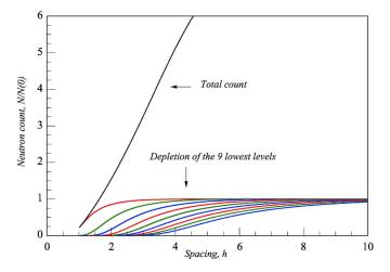
FIG. 10. (Color online) The neutron count N/N(0), Eq. (73), and individual depletions of the nine lowest energy levels, Eq. (74), as a function of the spacing between the walls *h* at  $\chi$ =0.15,  $\eta$ =r=0.01.
