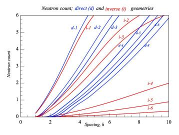
FIG. 14. (Color online) The depletion rates for direct (*d*; the scatterer is on the top) and inverse (*i*; the scatterer is on the bottom) geometries for  $\chi$ =0.15, *r*=0.015. The curves are marked by the ratio  $\eta/r$ =1, 2, 3, 4, 5, 6, 8 and by the geometry *d* or *i*.
