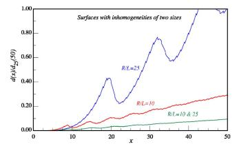
FIG. 13. (Color online) Diffusion coefficient for Gaussian inhomogeneities with R/L=10, R/L=25 and with the sum of inhomogeneities of both sizes. The curves are labeled by the value of R/L. All three curves are normalized by the value of d(R/L=25;x=50).
