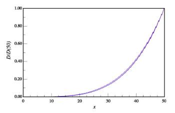
FIG. 2. (Color online) Normalized single-particle diffusion coefficient d(x)/d(50),  $x=L/\Lambda$  with artificially frozen mode coupling. The shapes of all five curves are identical irrespective of the type of inhomogeneities (Gaussian, exponential, or power law) and the value of R/L. Small sawtooth anomalies correspond to changes in the number of accessible minibands S(L), Eq. (31).
