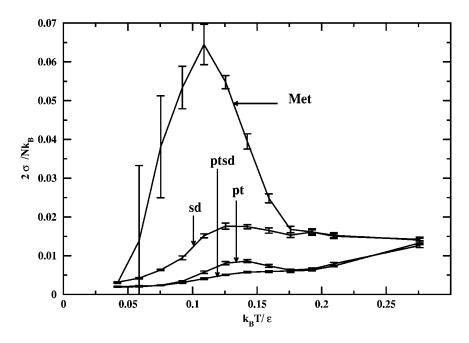
FIG. 2. Two standard deviations of the mean for the heat capacity per particle expressed in units of the Boltzmann constant as a function of the temperature expressed in units of  $\epsilon/k_B$ . The line marked Met represents the Metropolis data, the line marked sd represents the smart-darting data, the line marked pt represent the parallel tempering data, and the line marked ptsd represent the data when parallel tempering is combined with smart darting.
