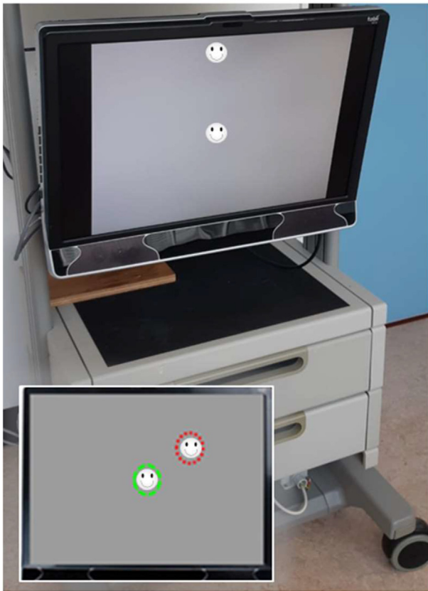
Figure 1. EMPP set up with a 24-inch display monitor integrated with an infrared eye-tracking device and a height/viewing angle adjustable surface housing. The inset picture shows an illustration of the smiley fixation target (circled with green dotted lines) and a peripheral smiley stimulus (circled with red dotted lines).
