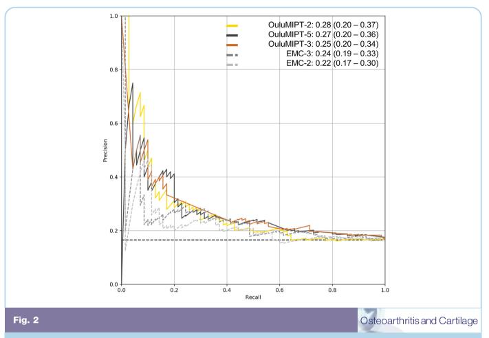
Precision-recall curves and respective area under the curve (PR AUC) values for the three algorithms with the highest PR AUC (*OuluMIPT-2*, *OuluMIPT-5*, and *OuluMIPT-3*) and for two reference models (*EMC-2* (age, BMI, and mild symptoms) and *EMC-3* (age, BMI, KL grade, and mild symptoms)).
