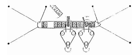
Since the jack-up rig is free standing there is no requirement to keep it in place. An anchoring system may be employed for safety reasons however, but this will not actually affect the location of the platform beyond the limit of the legs (BDM, 1988).
