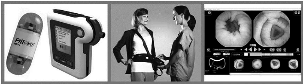
Supplementary figure 1. An image of the colon capsule and data recorder (left image), the sensor belt (image in the middle) and the Rapid™ software (right image).
