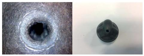
**Figure 1.** The synthetic papilla. **a**. Front view of the papilla. **b**. Close-up of the papilla, demonstrating the rubber with incorporated metal filaments.
