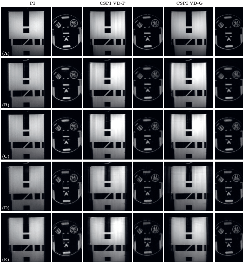
Figure 4.3: PD-weighted phantom images for 3D-FSE and 3D-GRASE with the proposed sampling patterns. Each row shows a different trajectory: (A) 3D-FSE with radial trajectory, (B) 3D-GRASE with SRE=0 (C) 3D-GRASE with SRE=1 (D) 3D-GRASE with SLCE 1 (E) 3D-GRASE with SLCE 2. Each column pair shows the different k-space grid: with a PI k-space grid, CSPI VD Poisson-disk undersampled k-space grid (VD-P) and the VD pseudo-random Gaussian undersampled k-space grid (VD-G) The sagittal and axial planes are shown for every k-space grid.
