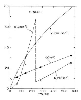
FIG. 6. Equilibrium values of various electron-swarm parameters in gaseous neon. The solid circles, open circles, and triangles are, respectively, the equilibrium values of  $\langle \varepsilon \rangle$ ,  $R_i$ , and  $V_d$ from the calculations of Kitamori *et al.* (Ref. 2). The dashed lines for the values of E/N below 35 Td correspond to extrapolated values of various parameters.
