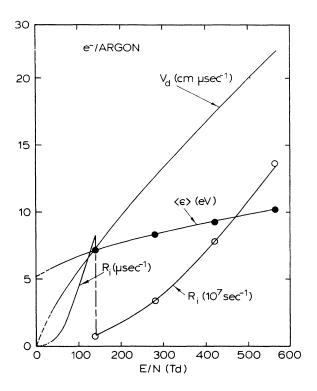
FIG. 9. Equilibrium values of various electron-swarm parameters in gaseous argon. The solid circles and the open circles are, respectively, the equilibrium values of  $\langle \varepsilon \rangle$  and  $R_i$  from the SST calculations of Sakai *et al.* (Ref. 10).
