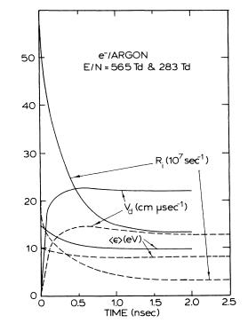
FIG. 7. Time dependence of various electron-swarm parameters in gaseous argon for E/N = 565 Td (solid curves) and 283 Td (dashed curves).
