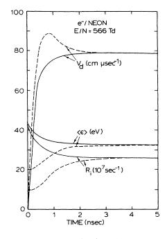
FIG. 4. Time dependence of various electron-swarm parameters in gaseous neon for E/N = 566 Td. The data corresponding to the solid curves and the dashed curves have initial average electron energy of 44 and 20 eV, respectively.
