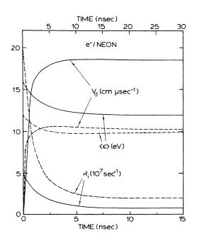
FIG. 5. Time dependence of various electron-swarm parameters in gaseous neon for E/N = 72 Td (solid curves) and 35 Td (dashed curves). The upper and lower time scales correspond to the 35- and 72-Td data, respectively.
