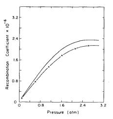
FIG. 2. Recombination rates for Kr<sup>\*</sup> and Kr<sup>\*</sup><sub>2</sub> with F<sup>-</sup> in Ar;—: Kr<sup>\*</sup>; ×—×: Kr<sup>\*</sup><sub>2</sub>.
