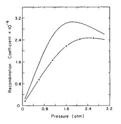
FIG. 1. Recombination rate in units of  $cm^3 sec^{-1}$  for  $Ar^*$  and  $Ar_2^*$  ions with F<sup>-</sup> in Ar as a function of the argon gas pressure;— $Ar^*$ ; ×—×:  $Ar_2^*$ .
