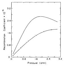
FIG. 3. Recombination rates for  $Ar^*$  and  $Hg^*$  with  $CI^-$  in  $Ar; -: Ar^*; \times - \times : Hg^*$ .
