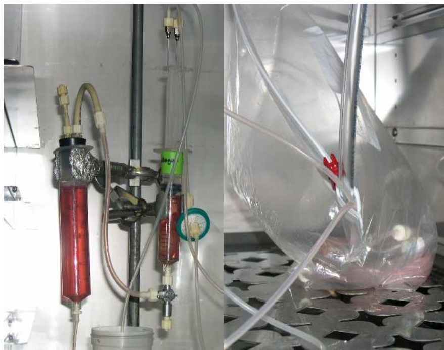
Figure 14: Bioreactor culture setup showing cell seeded scaffold, medium reservoir and oxygenator
