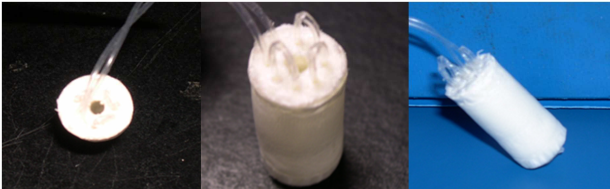
Figure 3: Top, front and angled view of chitosan scaffold embedded with gas permeable silicone tubing
