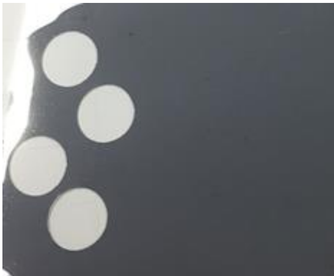
Figure 4-1 25 \mu m the thickness of the electrode
