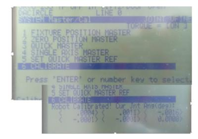
Figure 25: Calibrate on Teach Pendent of FANUC S-430 IW robot
