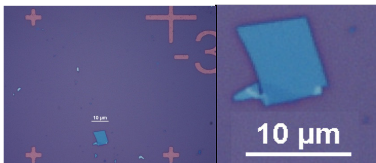
Fig.4.2.1 The left picture indicates the optical microscope image of 8.0 nm MoSe 2 sample with gold (Au) alignment marks and the right is close-up image of same sample on Si/SiO 2 substrate.
