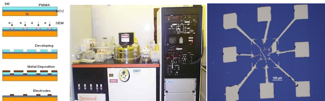
Fig.4.2.4 The schematic diagrams show the integrated processes with electron beam lithography and metal deposition, BJD 1800 e-beam metal evaporator and the device after gold deposition.
