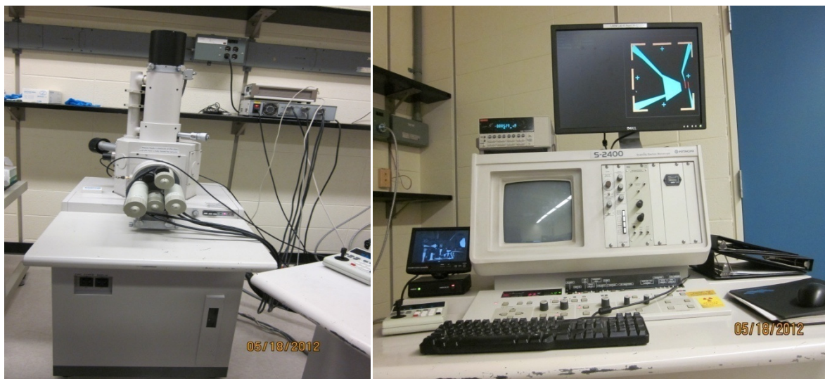
Fig.2.3.1 Scanning electron microscope (SEM) (Hitachi S-2400) set up for e-beam lithography.
