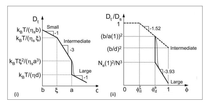
**FIGURE 2.1.1:** (i) Terminal particle diffusion coefficient  $D_t$  as a function of particles size d in entangled polymer solutions. (ii) Normalized terminal diffusion coefficient as a function of polymer concentration in entangled athermal polymer solutions.<sup>17</sup>
