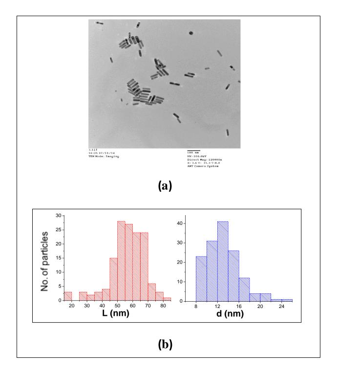
**FIGURE 4.5.1:** (a) TEM image of AuNPs deposited on carbon film magnified 800000×.JEOL-2010 FasTEM Transmission Electron Microscope (TEM) with a LaB6 filament working at 200
