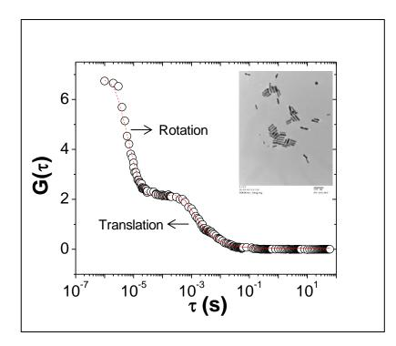
**FIGURE 5.3.1:** The cross-correlation function with fitting showing both the translational and rotational diffusions of the gold nanorods in phosphate buffer of pH 7.0. (Inset) Transmission Electron Micrograph of gold colloids collected using a JEOL 2010 TEM. The length and diameter of  $\approx$ 150 such particles are shown giving the average L $\approx$ 56 ± 4 nm and d  $\approx$ 13 ± 4 nm.
