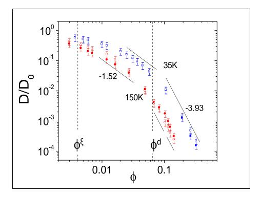
**FIGURE 4.3.3:** In log-log plot, the comparison of  $D(\phi)$  with scaling theory (Ref.17) is shown. The scaling predictions are solid line. The open symbols are translational diffusion and filled symbols are rotational diffusion. The two crossover volume fractions,  $\phi^{\xi}$  and  $\phi^{d}$  are also shown by the dashed lines. All the relevant parameters are listed in Table 4.3.2. The data for 5K was not plotted as they agree with hydrodynamic theory.
