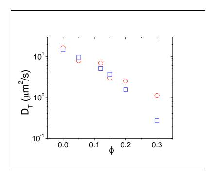
**Figure 6.5.3:** The theoretical translational diffusion coefficients using Stick theory (open circle) and the experimental value of translational diffusion coefficients (open square) from the CCF fitted with 2D Gaussian model are plotted as a function of Ludox concentrations.
