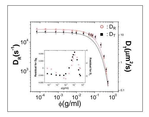
**FIGURE 5.3.3:** Rotational ( $D_R$ ) and translational ( $D_T$ ) diffusion coefficients of the nanorods are shown as a function of BSA concentration ( $\phi$ ). The error bars correspond to a minimum of five independent trials. The fitting is according to stretched exponential function. (Inset) The residual showed that systematic deviation from the fitting at all concentrations.
