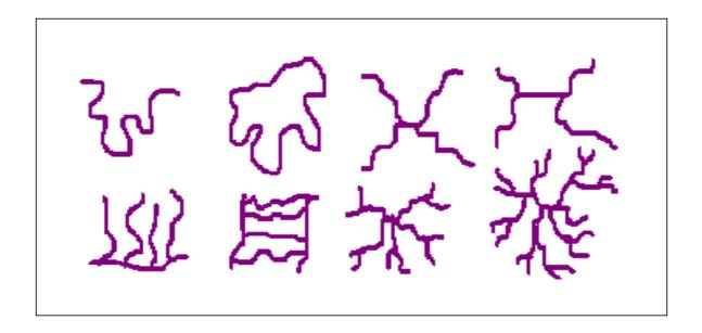
**FIGURE 1.2.1:** Examples of polymer architectures: linear, ring, star-branched, H-branched, comb, ladder, dendrimer, and randomely-branched.
