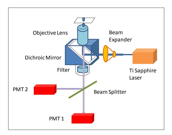
FIGURE 3.2.1: Two photon FCS set up for translational diffusion measurements.
