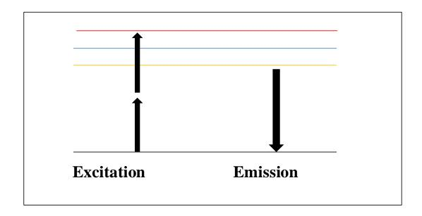
FIGURE 3.2.2: Diagram of two photon excitation.
