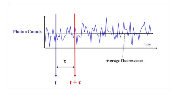
**FIGURE 3.1.1:** Fluctuation of fluorescence due to molecular motions and generation of autocorrelation function (ACF).
