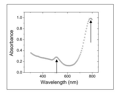
**FIGURE 4.1.1:** UV-vis spectra of AuNR in water (open circle) with two distinct peaks at 790 nm and 510 nm. The peak at 790 nm depends upon the aspect ratio of the rod.
