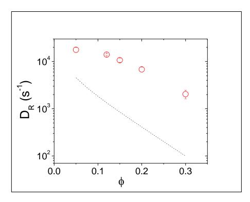
**FIGURE 6.5.4:** The rotational diffusion coefficients vs. volume fraction of Ludox. Experimental value of rotational diffusion coefficients were plotted as a function of ludox volume fractions (open circle). The dashed line (black) is fit using Pecora-Deutch theory with bulk viscosity  $\eta_b$  ( $\phi$ ), where we have considered that one monolayer of silica sphere will stick to rod surface due to electrostatic interaction i.e. L = 112 nm and d = 69 nm.
