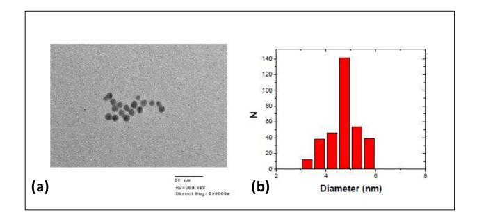
**FIGURE 7.1.2:** (a) TEM image of AuNPs deposited on carbon film magnified 800 000×. (b) A histogram obtained by measuring the diameters of AuNPs, where the average diameter measured is  $4.7 \pm 0.6$  nm.
