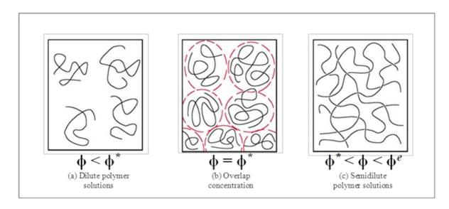
FIGURE 1.2.3: Different concentration regimes of flexible polymers.
