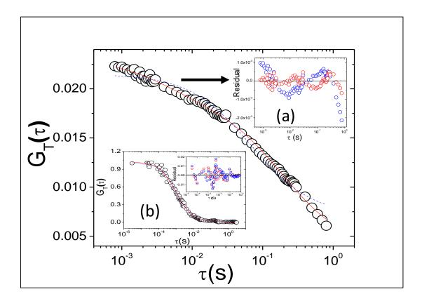
**FIGURE 6.3.1.1:** The imperfect fit with one-component translation diffusion coefficient is demonstrated. The solution is with Ludox volume fraction  $\approx 0.3$ . The dashed line through the points is one component fit ( $D_T \approx 0.3 \ \mu m^2/s$ ) and the solid line is two-component fit ( $D_{TI} \approx 5 \ \mu m^2/s$  and  $D_{T\perp} \approx 0.1 \ \mu m^2/s$ ). The corresponding residuals are shown in inset (a). Inset (b) showed
