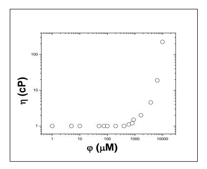
FIGURE 5.5.1: Viscosity vs. volume fraction plot for BSA in buffer (pH 7.0).
