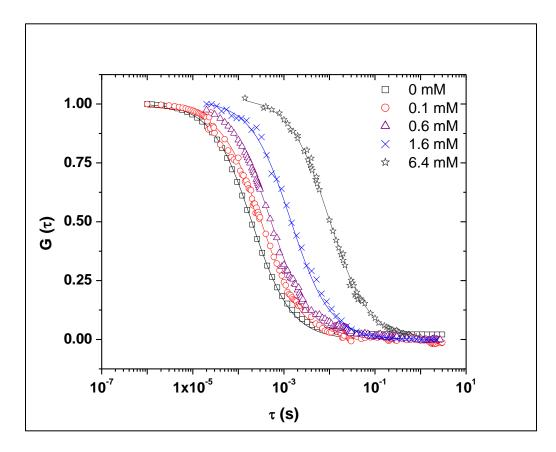
FIGURE 7.1.1: Normalized autocorrelation curves for AuNP (R= 2.5 nm) diffusing in BSA
