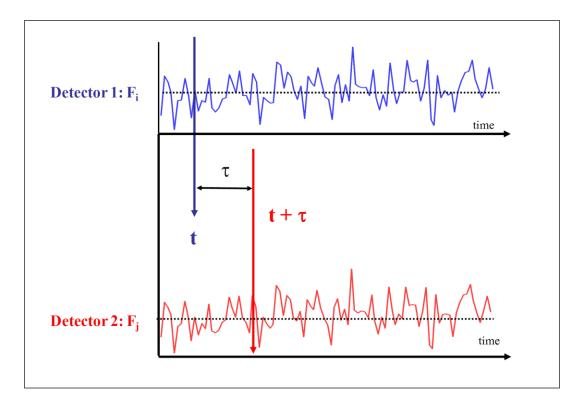
**FIGURE 3.1.2:** Fluctuation of fluorescence due to molecular motion and generation of cross-correlation function (CCF).
