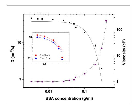
**FIGURE 7.1.3:** Diffusion coefficient of R = 2.5 nm AuNPs as a function of protein concentration. The inset shows the measured diffusion for 5 and 10 nm AuNPs at higher concentrations of BSA. Also shown (stars) viscosity as a function of BSA concentration.
