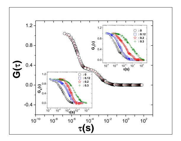
**FIGURE 6.2.1:** Cross-correlation function,  $G(\tau)$  with fitting as described in the text showing both the translational and rotational diffusion of the gold nanorods in water (main figure). Rotational (inset bottom) and translational (inset top) cross-correlation curves were shown separately for different volume fractions of Ludox as indicated in the caption. The nanorods concentration was kept at about ~ 1 pM. The imperfect fit of the translation curves are described later.
