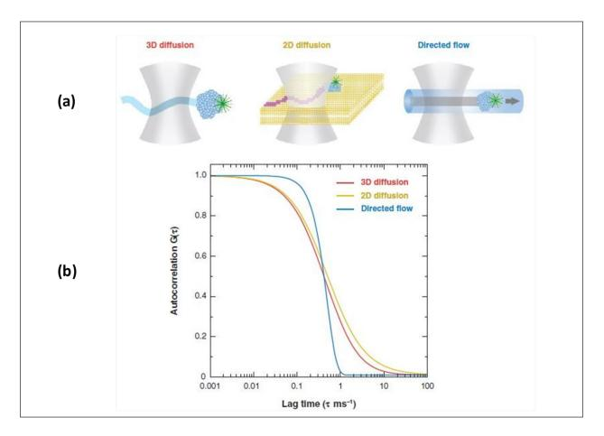
**FIGURE 3.1.3:** (a, b): Model autocorrelation curves for different kinds of particle motion: free diffusion in three dimensions (red), free diffusion in two dimensions, e.g., for membrane-bound molecules (yellow) and directed flow (Cyan).<sup>80</sup>
