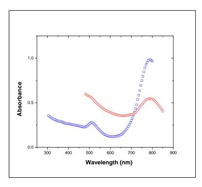
**FIGURE 6.5.2:** UV-vis spectra of AuNR in water (open square) with two distinct peaks at 790 nm and 510 nm. The peak at 790 nm depends upon the aspect ratio of the rod. UV-vis spectra for AuNR in Ludox (open circle) for the highest volume fraction of silica spheres with peak at 787 nm.
