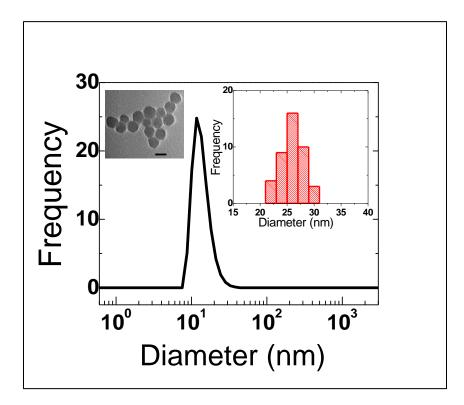
**FIGURE 6.5.1:** Size distribution of silica nanoparticle obtained from dynamic light scattering (DLS) measurement with a mean diameter 24 nm, and showed no sign of any agglomeration; Left inset: shows a representative TEM micrograph with 20 nm scale bar; Right inset: histogram of size distribution obtained from TEM with mean diameter of  $26 \pm 3$  nm. The average size provided by the manufacturer was 22 nm.
