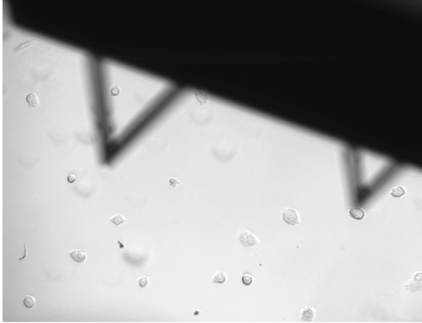
Figure 6.7: It shows the field of view where unfunctionalized DNP-C cantilever is scanning on top of a BPH1 scr cell
