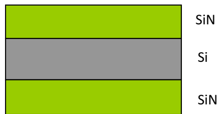
Fig. A.7. Schematics to show SiN layers on front and back of Si wafer
