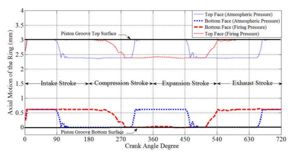
Fig. 4-33 Ring axial position within the piston groove.
