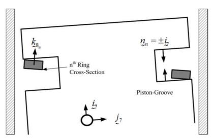
Fig. 2-10 Schematic illustrating the normal vectors to the ring and the groove surfaces.
