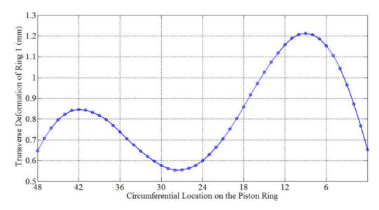
Fig. 4- 22 In-plane transverse deformation of the first compression ring at  $295^{\circ}$  CAD.
