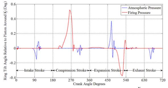
Fig. 4- 32 Tilt angle of the ring with respect to the piston around the  $\frac{K}{2}$  direction.
