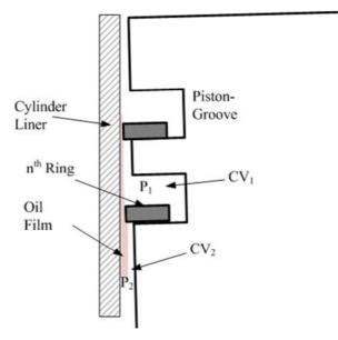
Fig. 2- 8 Schematic illustrating pressure notations for control volumes surrounding the rings.
