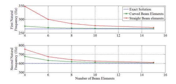
Fig. 2-5 Convergence rate of the curved beam finite element model of the ring.
