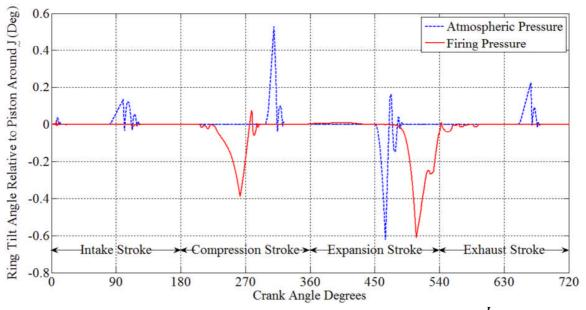
Fig. 4- 31 Tilt angle of the ring with respect to the piston around the  $\frac{J}{2}$  direction.
