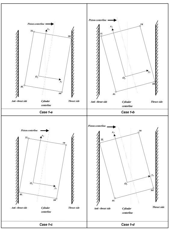
Fig. 2- 2 Piston-liner interactions through a single point contact [58].
