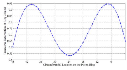
Fig. 4- 26 In-plane transverse deformation of the third compression ring at 295° CAD
