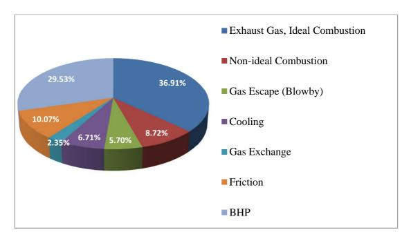
Fig. 1-1 Percentage distribution of the fuel energy between BHP and other sources of power losses for Diesel engine operating at 20% load (data taken from Ref. [1])
