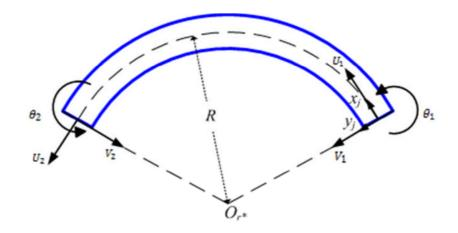
Fig. 2- 4 Curved beam Finite element with nodal coordinates
