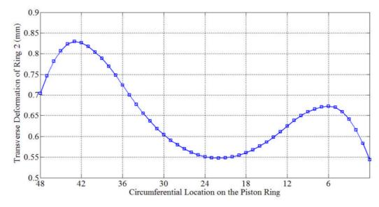
Fig. 4- 24 In-plane transverse deformation of the second compression ring at  $295^{\circ}$  CAD.
