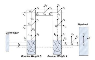
Fig. 2-1 Schematics of the crankshaft, connecting-rod, and piston.
