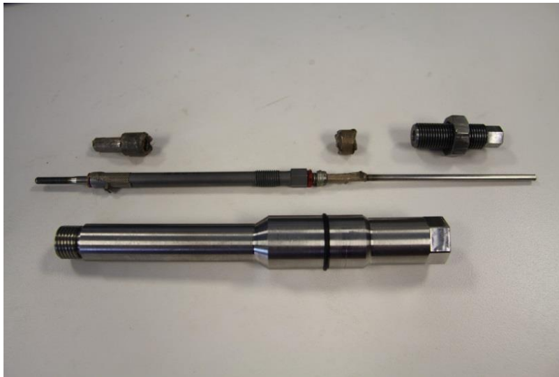
Figure 3.7: Ion Current Glow Plug with Brazed Rod
