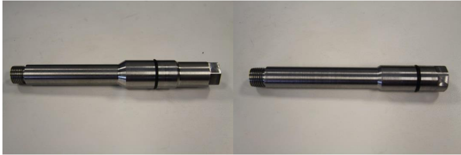
Figure 3.5: Pressure Transducer Sleeve (Left) and Glow Plug Sleeve (Right)
