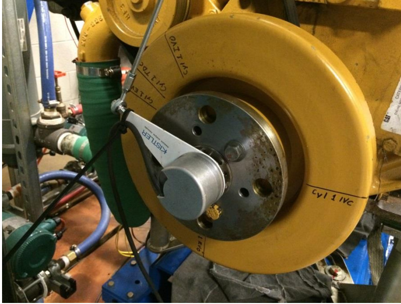
Figure A. 2: Labeling of Injection Timings Events on Crankshaft Pulley
