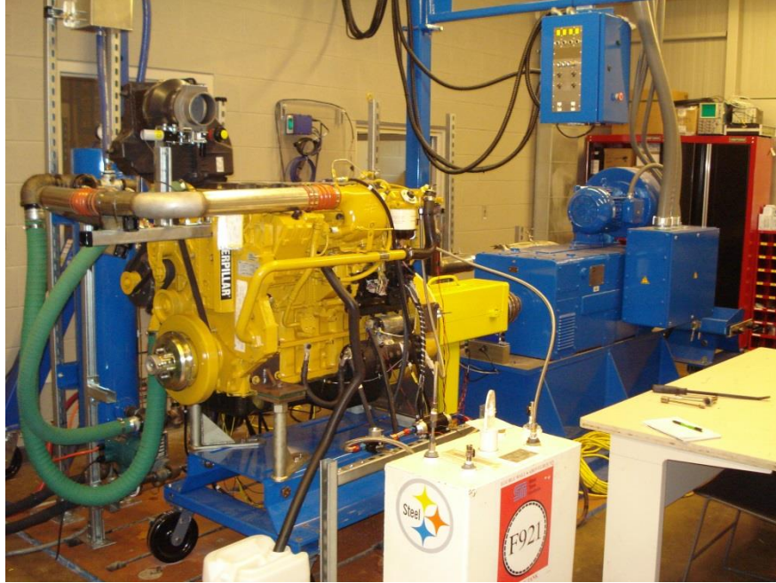
Figure 3.1: Engine and Dynamometer Setup
