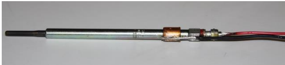
Figure 3.6: Ion Current Glow Plug with Attached Wires
