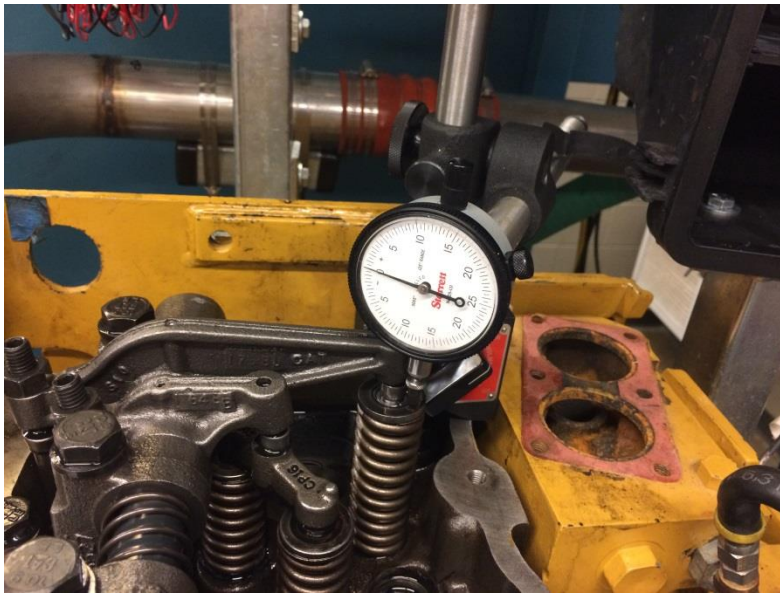
Figure A. 1: Position of Dial Indicator to Measure ValveTimings
