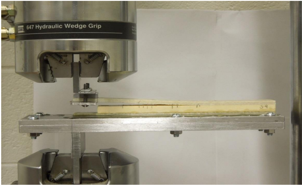
Figure 5.1: T-Peel test setup and SCB sandwich specimen.
