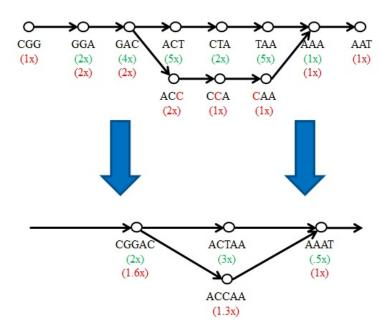
Figure 2.4: Colored de Bruijn graph condensation stage is presented. The colored coverage of the condensed node is the average of the colored coverage of all the nodes in the path.
