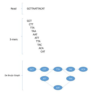
Figure 2.1: The construction of de Bruijn graph for a given read with k = 3 is illustrated. Ten 3-mers are generated for the 12 character long sequencing read. Each 3-mer is represented by a node in the graph. Two consecutive 3-mers are connected by a directed edge. A node can represent more than one loci if the sequence of all representative 3-mers are equal (node TTA represents two loci).
