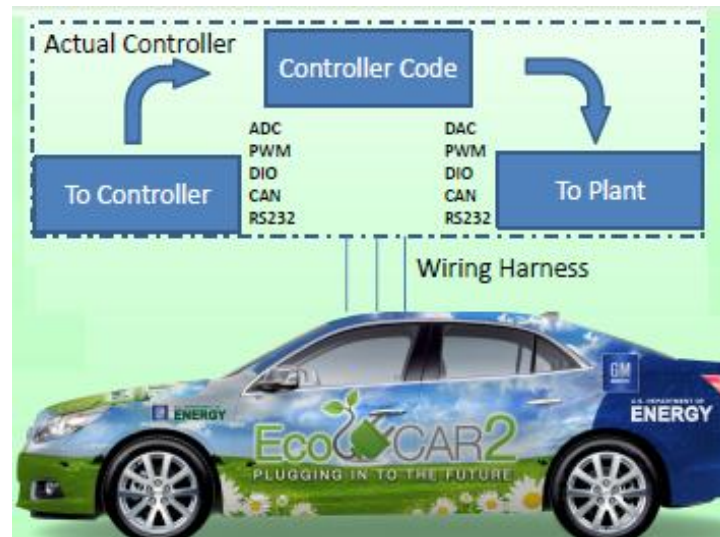
Figure 1-4. VIL (Vehicle-in-the-loop) Data Flow [9]
