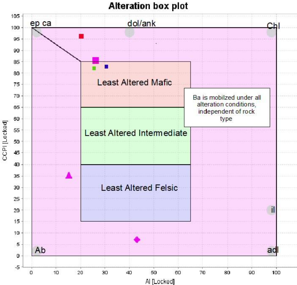
Figure 76 Alteration Box Plot considering barium of the Southwest Bristol Porphyry, Thunder Creek Syenite, Holmer Porphyry, and Tonalite-Melteigite (Alkalic intrusive). Results indicate that Ba is mobilized under all alteration conditions. Size and color correspond to Ba concentration, Blue < 200 ppm, Green – 200 to 300 ppm, Red – 300 to 1,000 ppm and Purple >1,000 ppm. Southwest Bristol – Upright Triangle, Thunder Creek Syenite - Diamond, Holmer Porphyry - Inverted Triangle, and Tonalite-Melteigite (Alkalic intrusive) - Square. Modified from Large et al., 2001.
