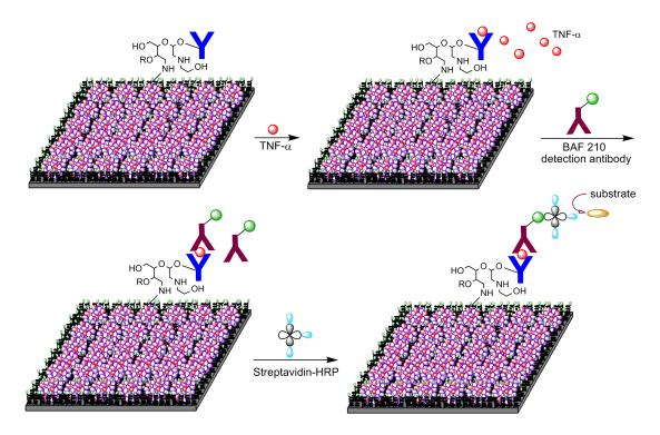
Figure 31. Schematic representation of TNF- $\alpha$  assay using dendrimer modified ELISA plate.
