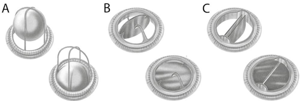
Figure 2 | Opening and closing mechanism of the three main types of mechanical heart valves. (A) Starr-Edwards "ball-in-cage" valve. (B) Medtronic-Hall tilting disc valve. (C) St. Jude Medical bi-leaflet valve. Image (modified) courtesy of Jaron D et al. The Body Synthetic .
