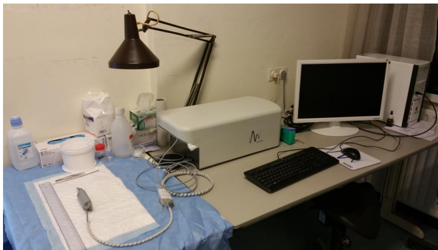
Figure 1. First prototype: fiber optic needle probe Raman instrument.
