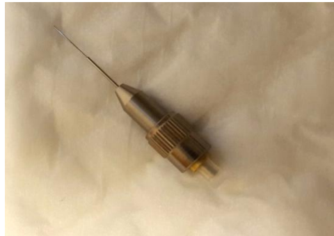
Figure 3. Example of a disposable 50 \mu\text{m} -core fiber-optic needle (art photonics GmbH, Germany).
