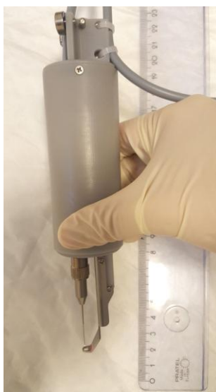
Figure 2. Prototype fiber optic Raman needle probe.
