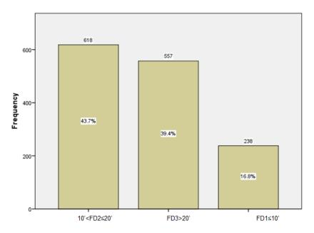
Figure 36: Frequency analysis for fall distance among roofers
