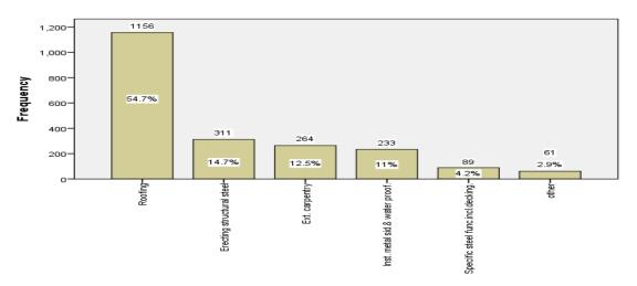
Figure 22: Frequency analysis for construction operation prompting fall
