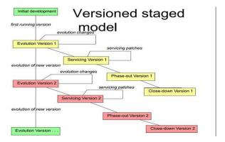
**Figure 2-8:** The versioned staged model of software
