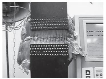
Figure 1 Photograph of the test setting used. The sutured abdominal wall is fixed in the tensile testing machine and is pulled apart at a constant rate of 10 mm/min.
