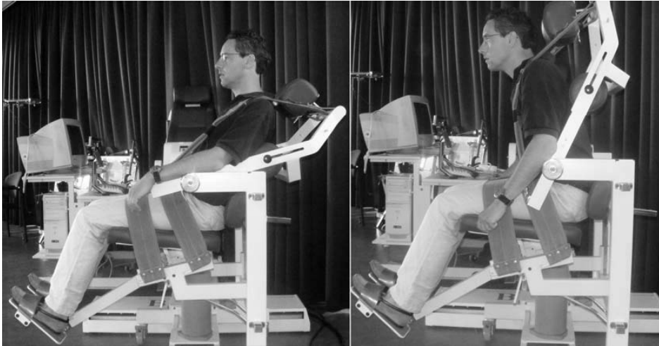
Fig.1 . Set-up of Biodex® isokinetic dynamometer
