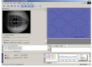
**Figure 9:** A screen image of the interface of the eye tracker used in the present thesis. The left eye of the subject is being monitored during the eye movement experiment. The position and the timing of the eye movement can be monitored on line. The data could be recorded for further analyses.
