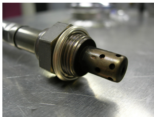
Figure 3.5. Horiba Mexa-700 \lambda display and sensor
