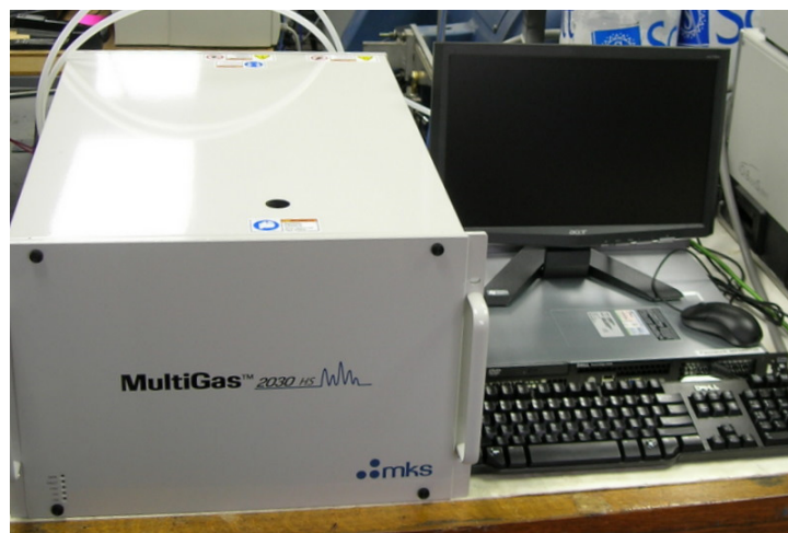
Figure 3.7. MKS Multi-Gas 2030 FTIR exhaust gas analyzer
