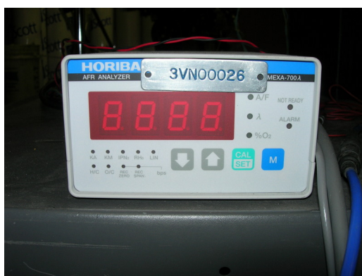
Figure 3.5. Horiba Mexa-700 \lambda display and sensor
