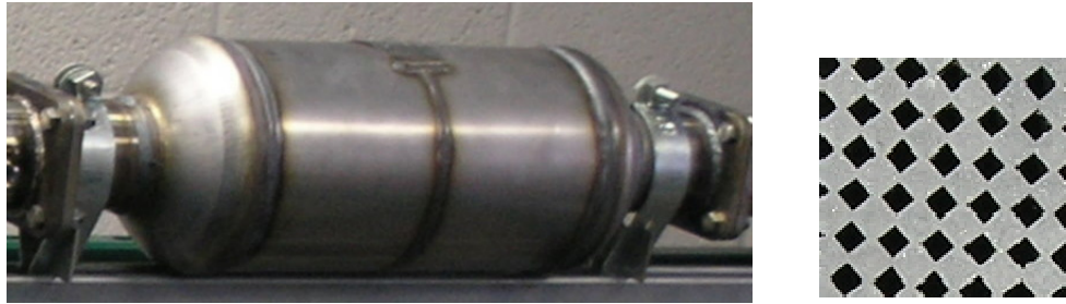
Figure 3.15. Diesel particulate filter and inside catalyst
