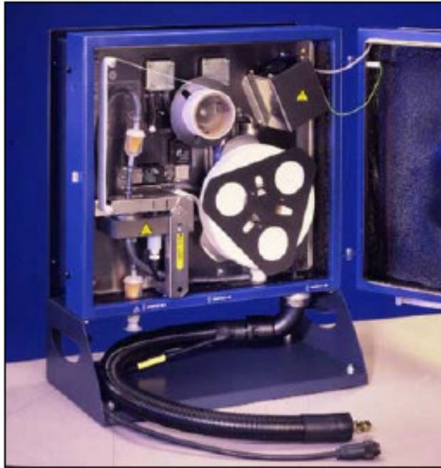
Figure 3.8. Interior of AVL 415S Smoke Meter
