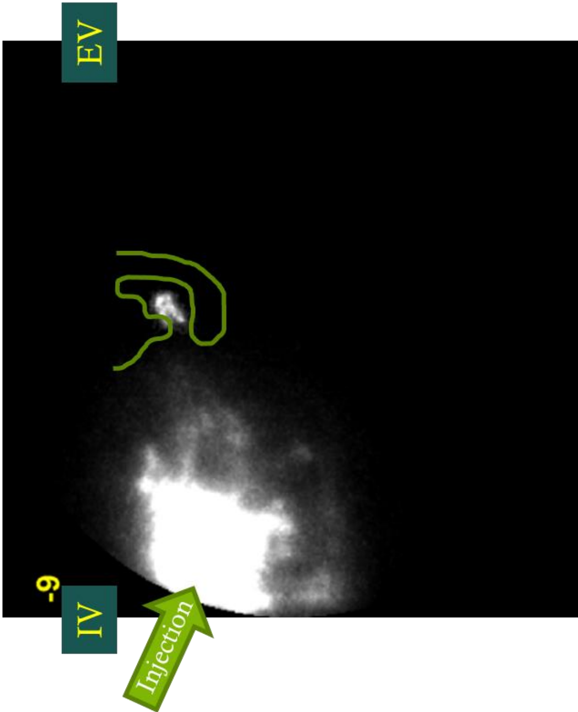
Figure 4.8.5 (b) Pre-ignition image (1° after ST)
