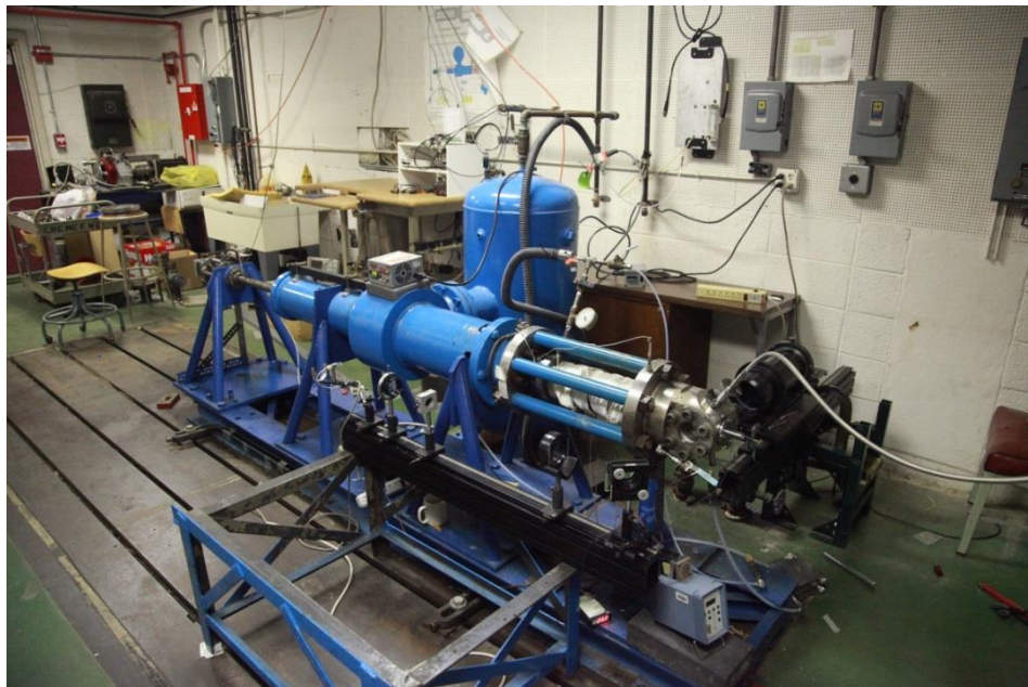
Figure D-4 RCM system
