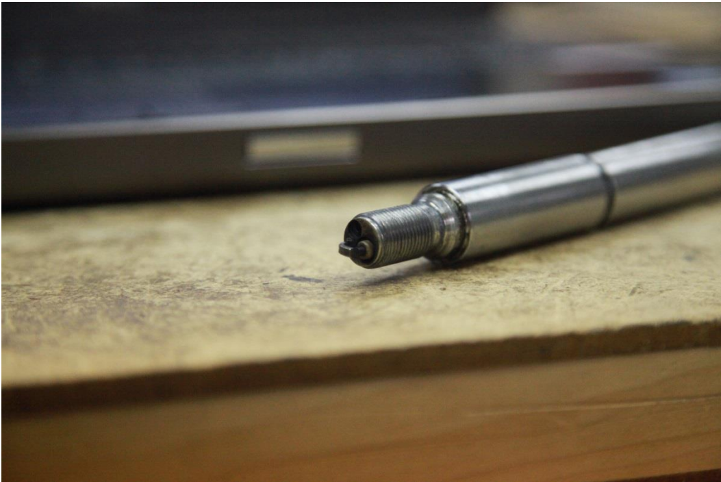
Figure 3.2.3 (b) sOAE devices: in-spark-plug pressure transducer
