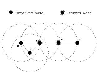
Figure 3.8: Initial Marking Process on a sample ad hoc wireless network<sup>b</sup>
