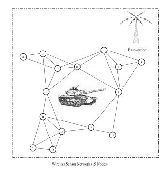
Figure 3.14: Wireless sensor network after neighbor discovery stage
