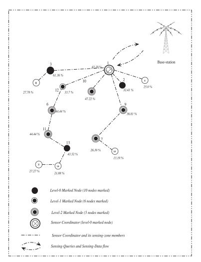
A Sensing zone with sensor-coordinator and its members (unmarked nodes and CDS nodes)
