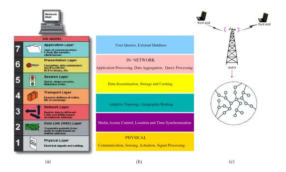
Figure 1.6: (a) Traditional OSI model, (b) Layered communications architecture for sensor networks<sup>c</sup>, and (c) Typical sensor network infrastructure.
