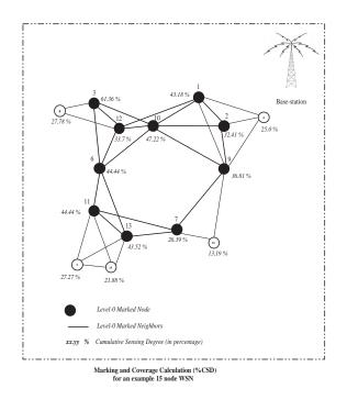
Figure 3.15: Wireless sensor network after the marking stage
