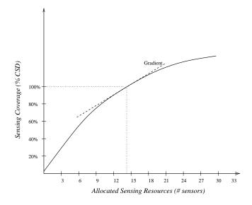
Figure 4.8: Marginal benefit to applications desiring sensing coverage
