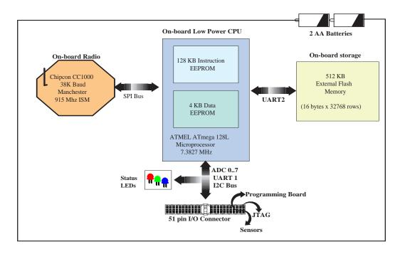
Figure 1.3: Basic architecture of a MICA2 sensor platform
