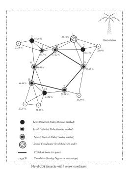
Figure 3.16: CDS hierarchy with sensor coordinator
