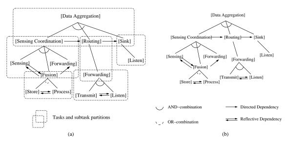
Figure 4.3: Data Aggregation: (a) Hierarchical decomposition and (b) Task Graph
