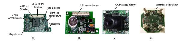
Figure 1.4: Multi modal Sensor Boards<sup>a</sup>
