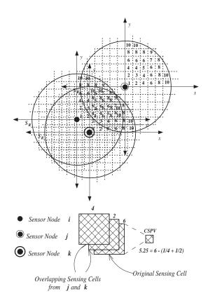
Figure 3.12: Calculating Cumulative Sensing Coverage
