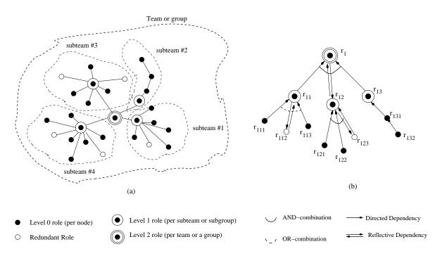
Figure 4.13: Monitoring Role failures: (a) Hierarchical Role-network organization and (b) Dominating roles acting as monitors for roles at lower level.
