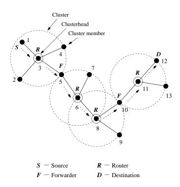
Figure 1.10: Cluster organization limits the role assignment of every cluster member to a forwarder and a clusterhead to a router.
