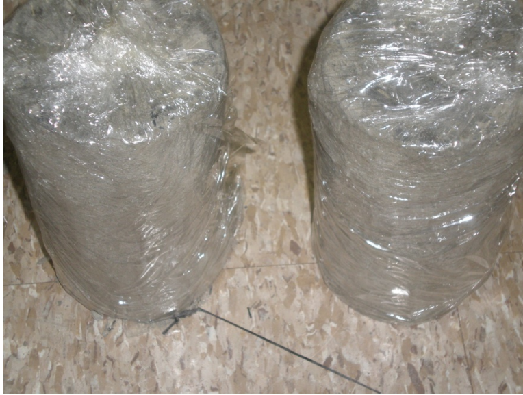
Figure 8.8: Plastic sheets curing for column specimens
