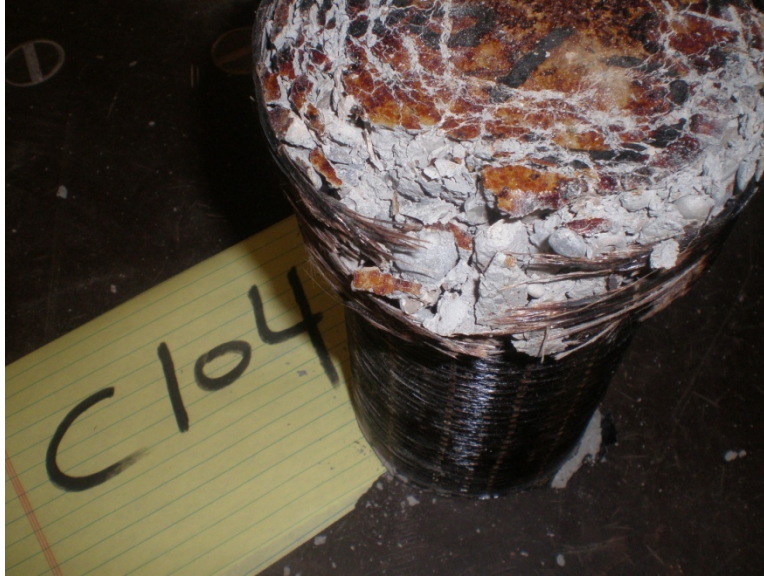
Figure 6.156: FRP rupture, C104 -180°C, 100% RH
