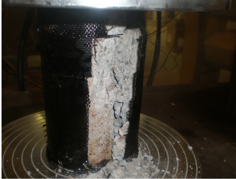
Figure 6.138: FRP rupture of C93-180°C, 100 cycles
