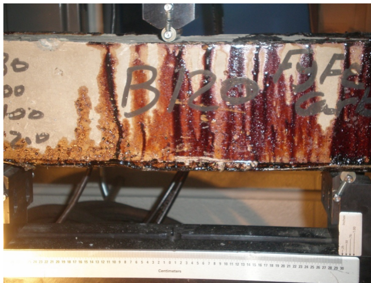
Figure 6.142: Flexural load test, B120
