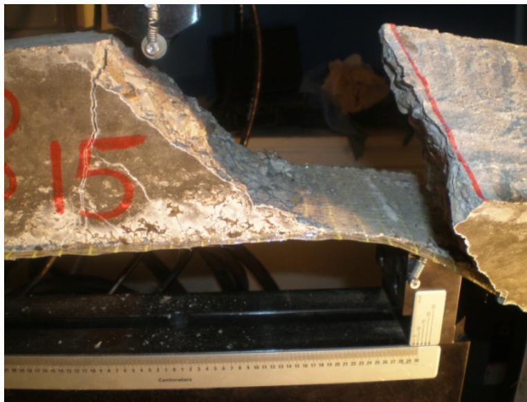
b) Shear failure and FRP delamination, B15
