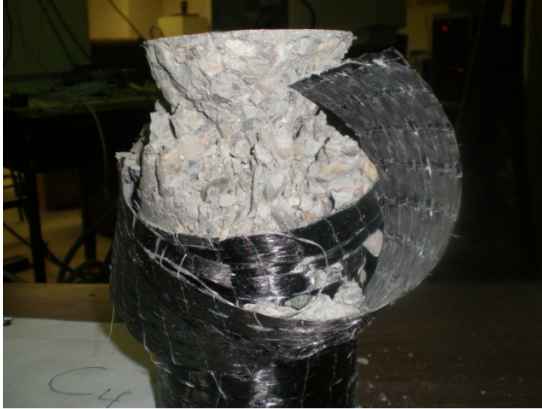
Figure 6.81: Compression test- FRP ruptures, C4
