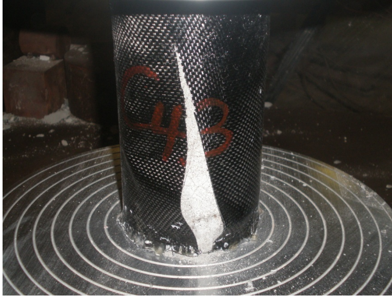
Figure 6.132: FRP rupture of C38-100°C, 40cycles
