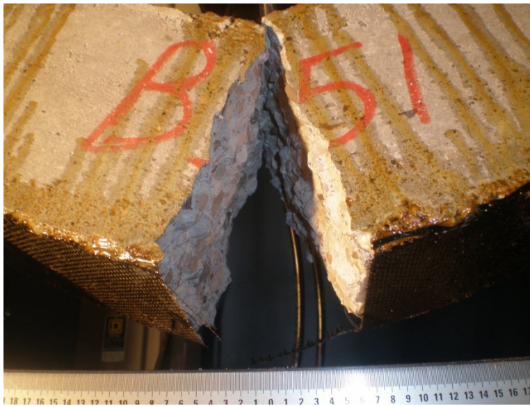
Figure 6.115: Typical mode of failure “FRP rupture” for concrete beam specimens (B51) at 100°C and 250 cycles
