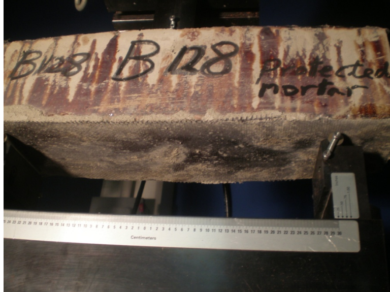
Figure 8.9: Center-point flexural load test, B128
