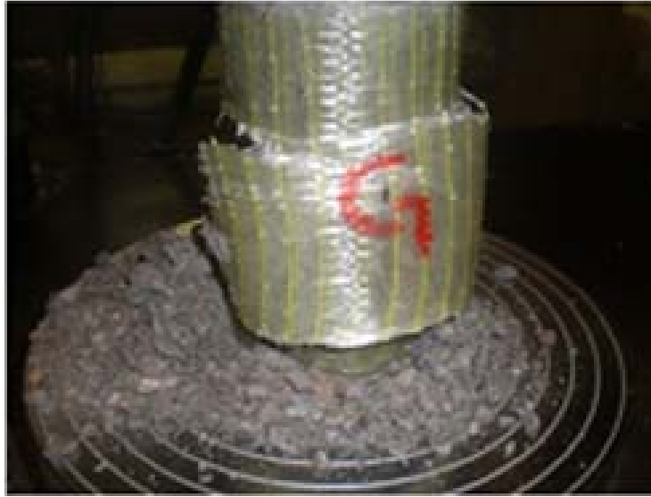
Figure 6.87: Concrete crushing and GFRP rupture of C7, opposite side of Fig 6.86
