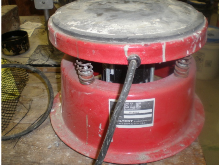
a) Concrete external vibrator was used for column specimens (model # AP-910-A)
