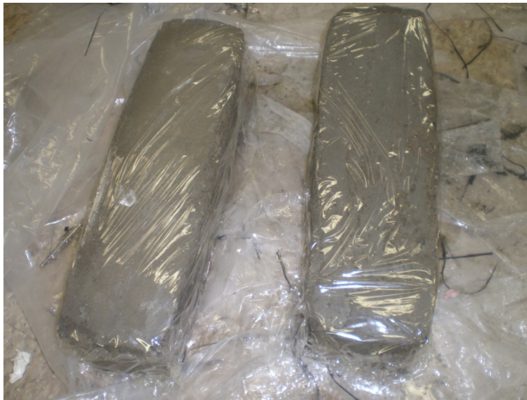
Figure 8.7: Wet plastic curing for beam specimens
