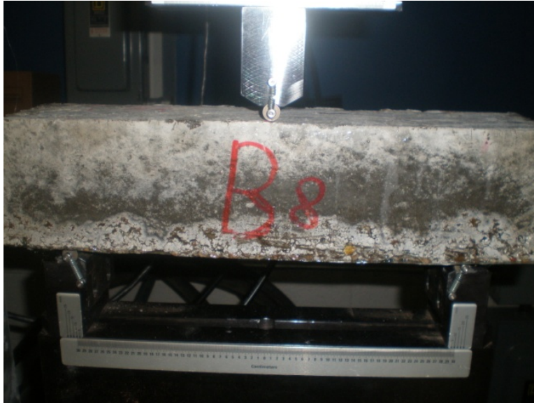
Figure 6.60: Beam specimen B8 strengthened by Sika GFRP
