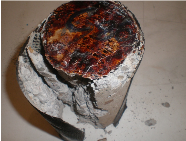
Figure 6.136: FRP rupture of C86-180°C, 40 cycles
