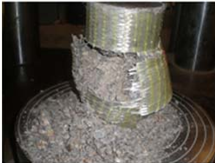
Figure 6.86: Concrete crushing and GFRP rupture of C7
