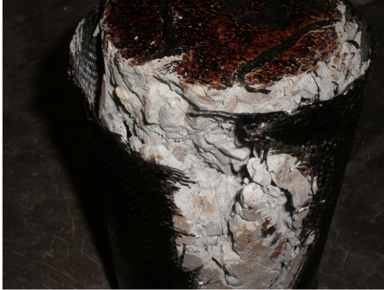
Figure 6.140: FRP rupture of C95-180°C, 250 cycles
