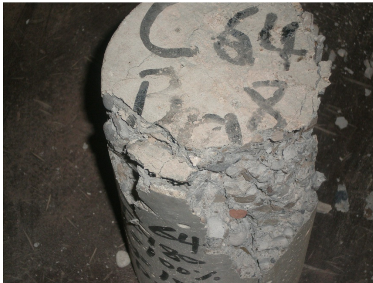
Figure 6.23: Compression failure of specimen C64 -180°C
