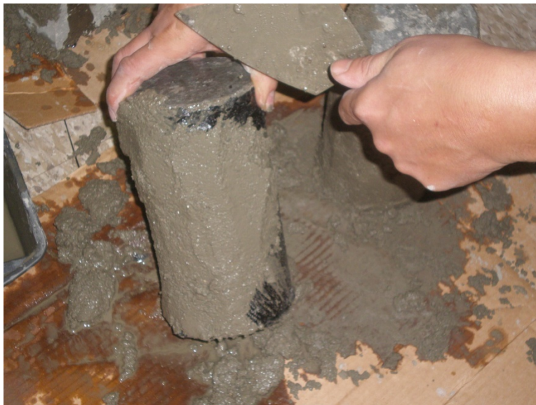
Figure 8.5: Protection procedures for column specimen
