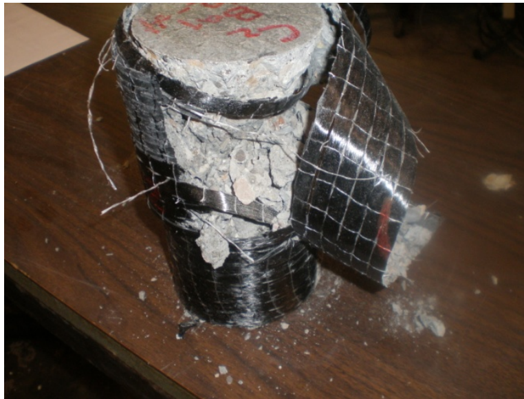
Figure 6.80: Compression test- FRP ruptures, C2
