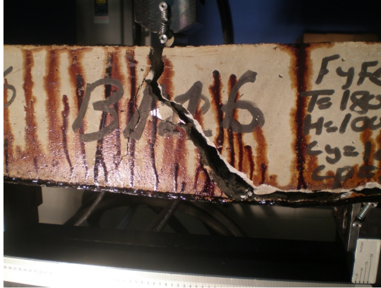
Figure 6.146: Concrete shear crack and FRP delamination of B116-180°C, 100% RH
