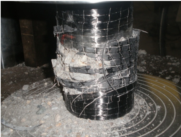
Figure 6.82: Compression test- FRP ruptures, C5
