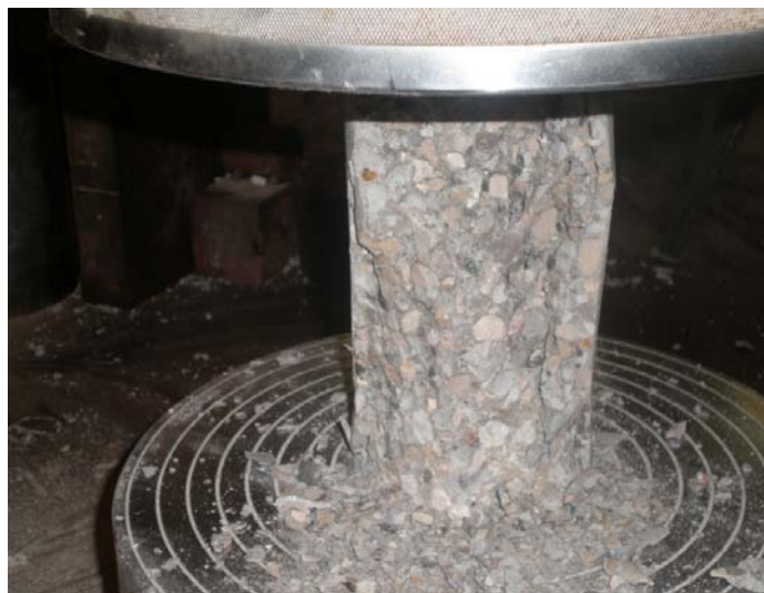
Figure 6.17: Concrete splitting failure of C1
