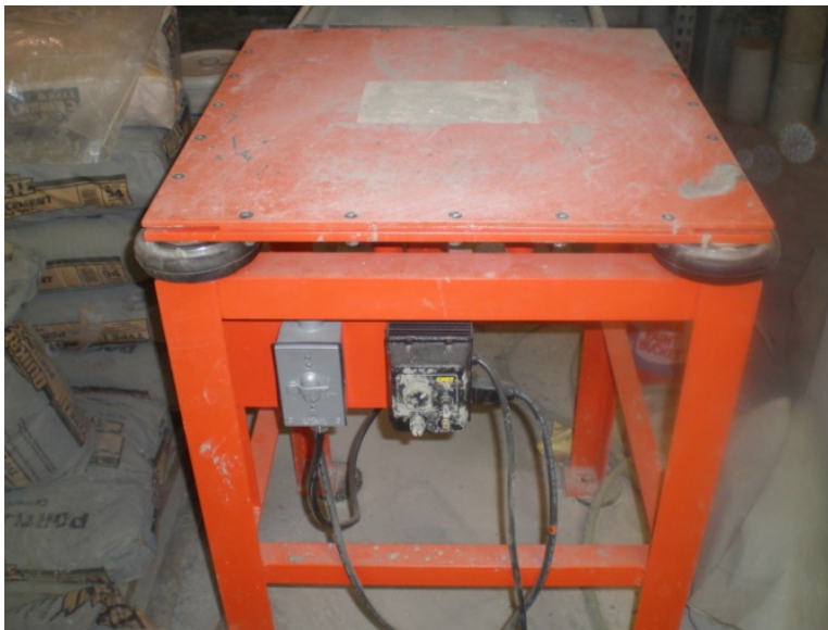
b) Concrete external vibrator was used for beam specimens
