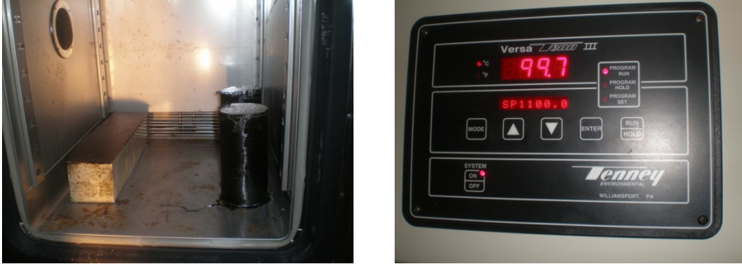
Figure 3.20: Temperature/Humidity environmental chambers
