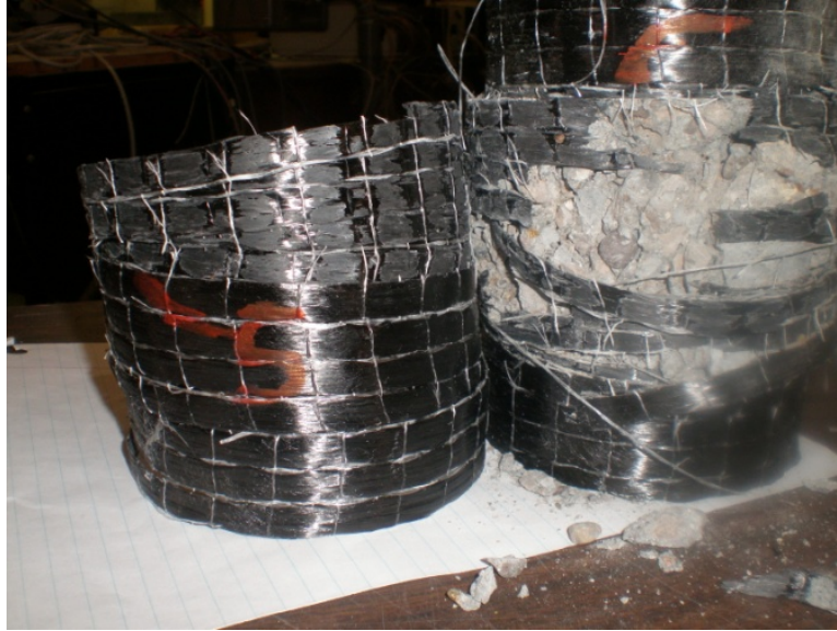
Figure 6.83: Delamination failure between two CFRP layers, a large portion of the top layer (on left) was ejected from the specimen at the time of failure, C5
