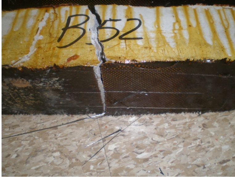
Figure 6.116: Typical mode of failure “FRP rupture” for concrete beam specimens (B52) at 100°C and 625 cycles
