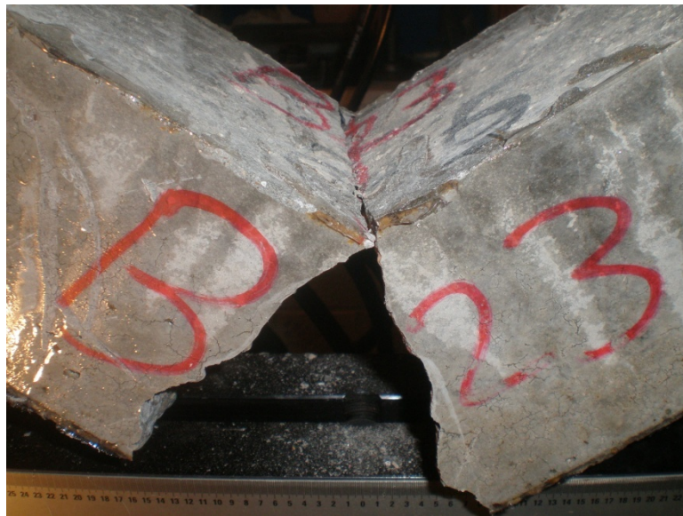
Figure 6.110: Concrete flexural failure and FRP rupture of B23
