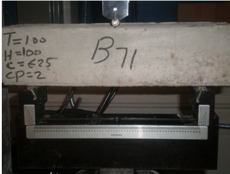
Figure 6.5: Concrete beam subjected to flexural load test
