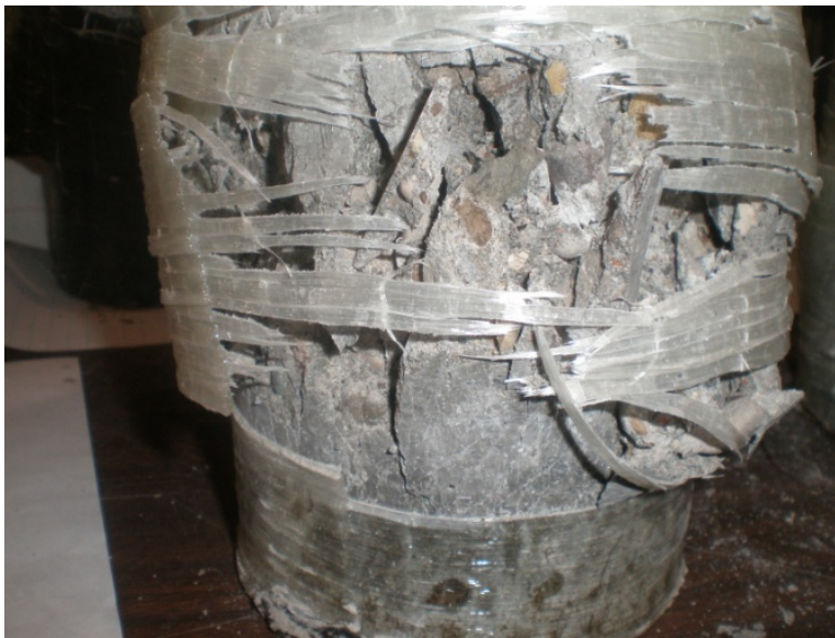
b) GFRP rupture and strips rip of C9 on the opposite side to (a)
