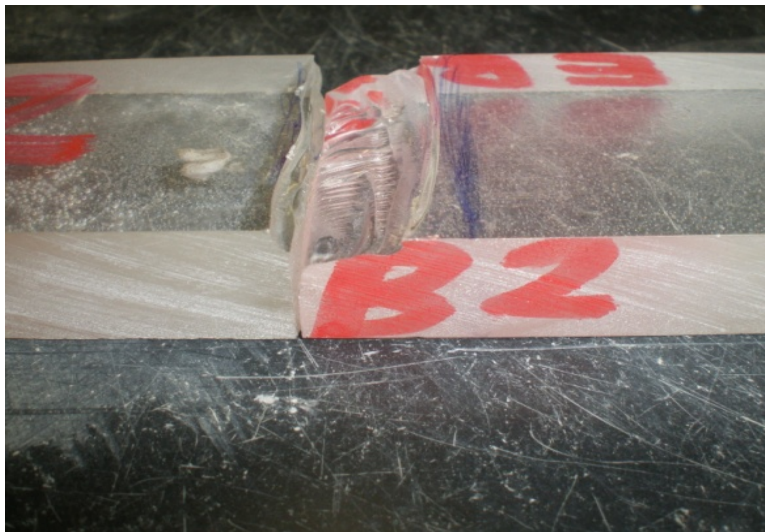
Figure 6.31: Flexural failure of the epoxy beam (EB2) at 40 Cycles
