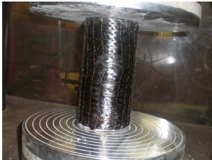
Figure 6.150: Compressive strength test, C68 (Fyfe CFRP)
