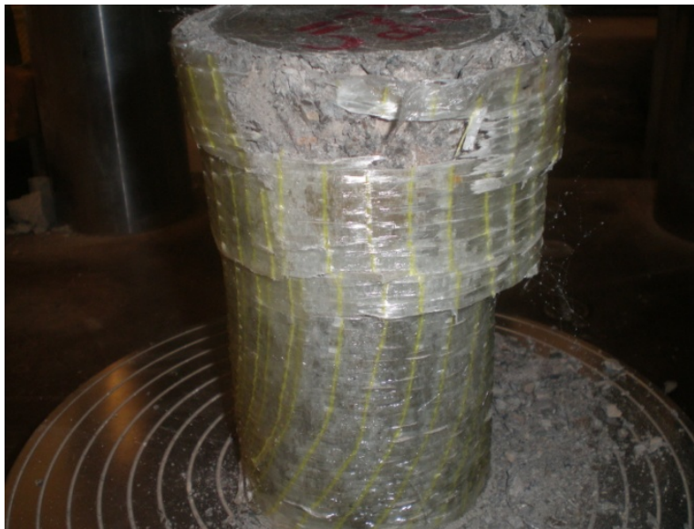
Figure 6.88: Concrete crushing and FRP rupture of C11
