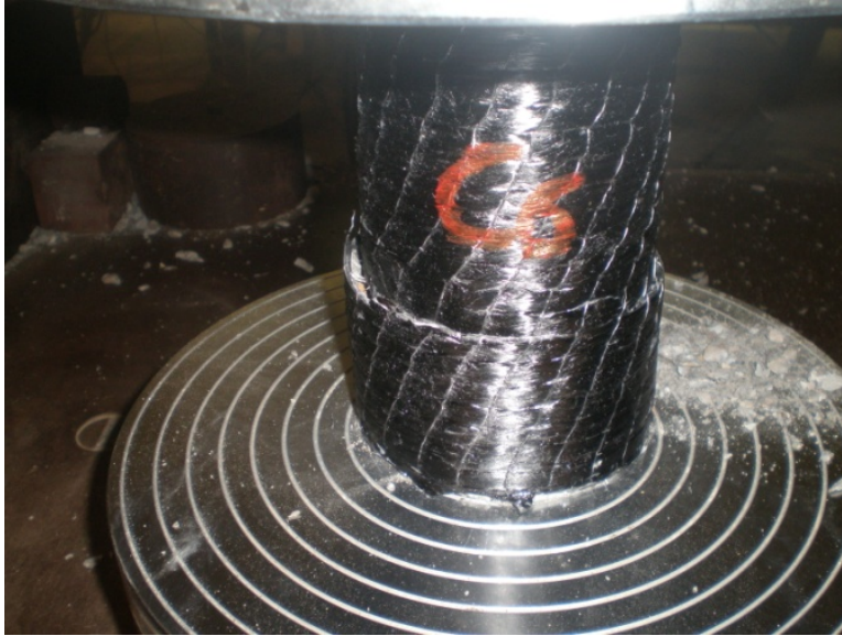
Figure 6.107: Hoop direction FRP rupture around the perimeter of the specimen, C6
