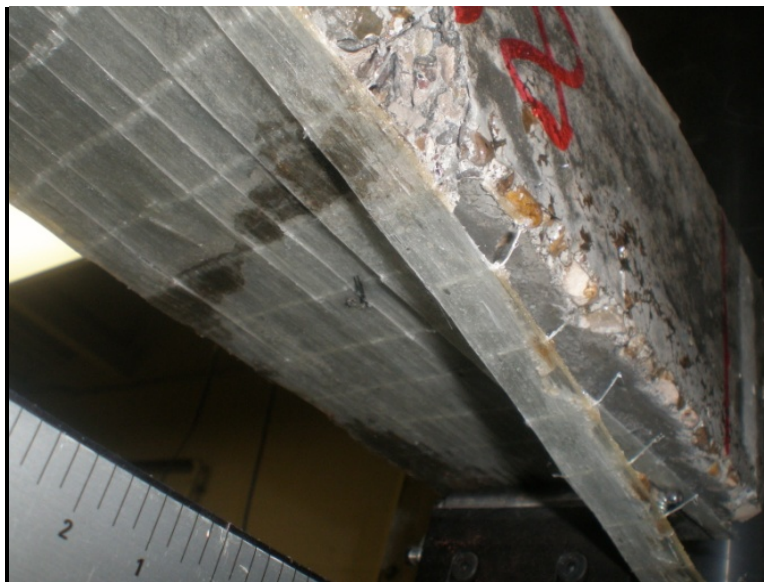
b) FRP Strips rip at the time of failure, B8
