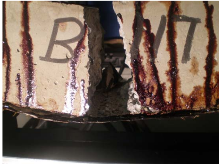
Figure 6.145: Concrete flexural crack and FRP delamination of B117-180°C, 100% RH
