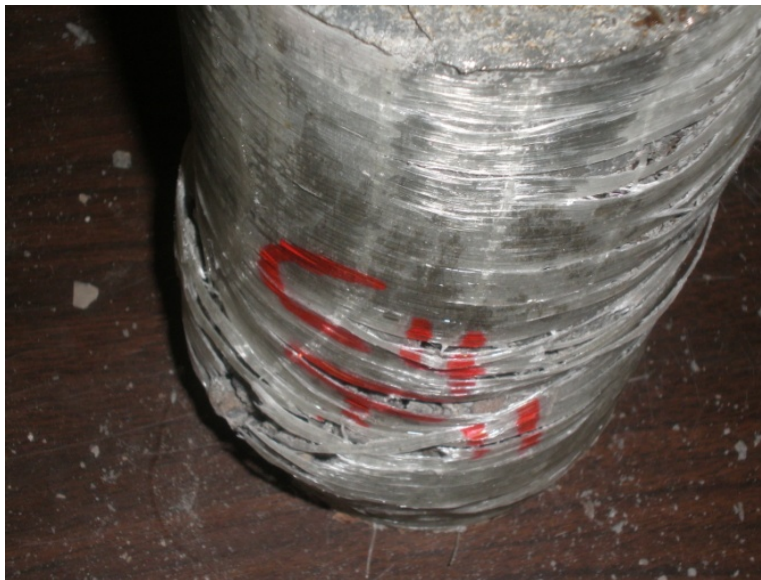
b) GFRP rupture and strips rip of C4T1
