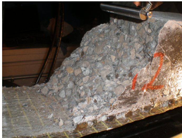
b) Shear failure and FRP delamination, B12
