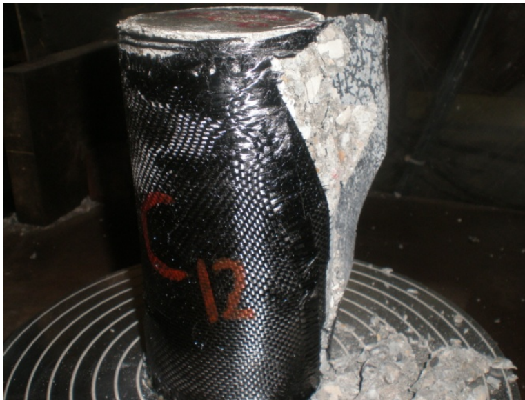
Figure 6.103: Concrete crushing and FRP rupture along the height of the specimen, C12
