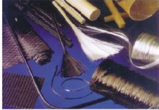
Figure 1.1: Common glass and carbon fibers and FRPs used in structural engineering [16]
