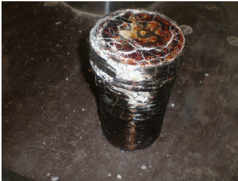
Figure 6.152: FRP rupture, C68 -180°C, 100% RH
