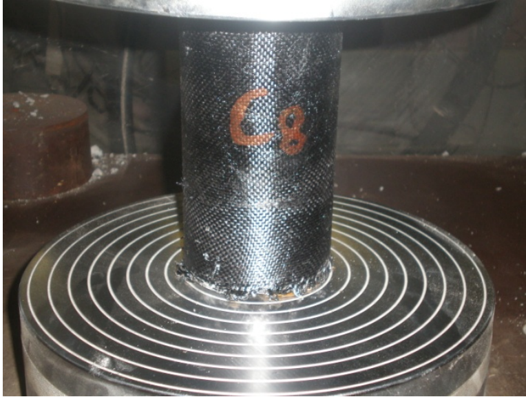
Figure 6.100: Compression strength test for column specimen strengthened by Sika CFRP and Fyfe epoxy
