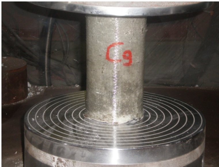
Figure 6.68: Compressive strength test for C9 specimen wrapped by Sika GFRP
