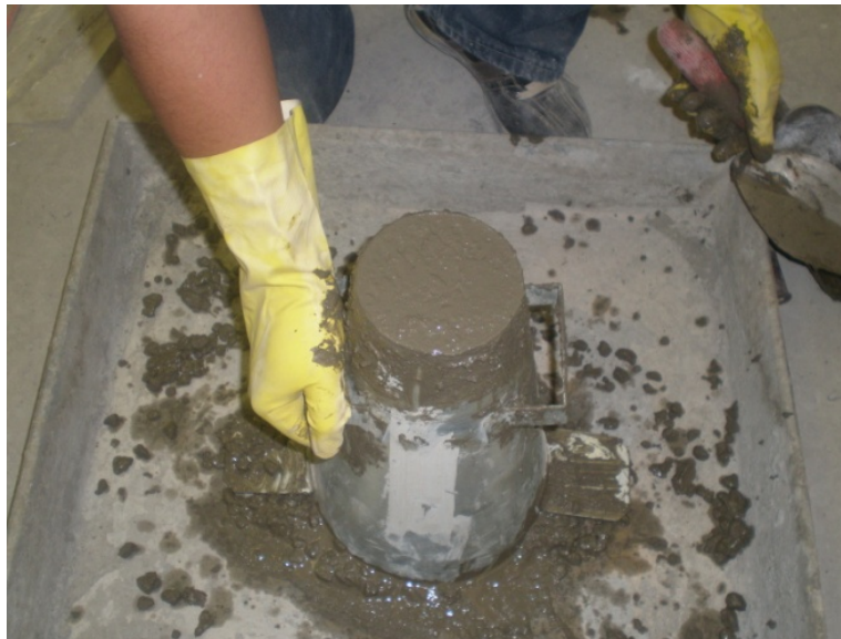
a) Slump test cone filled out by concrete
