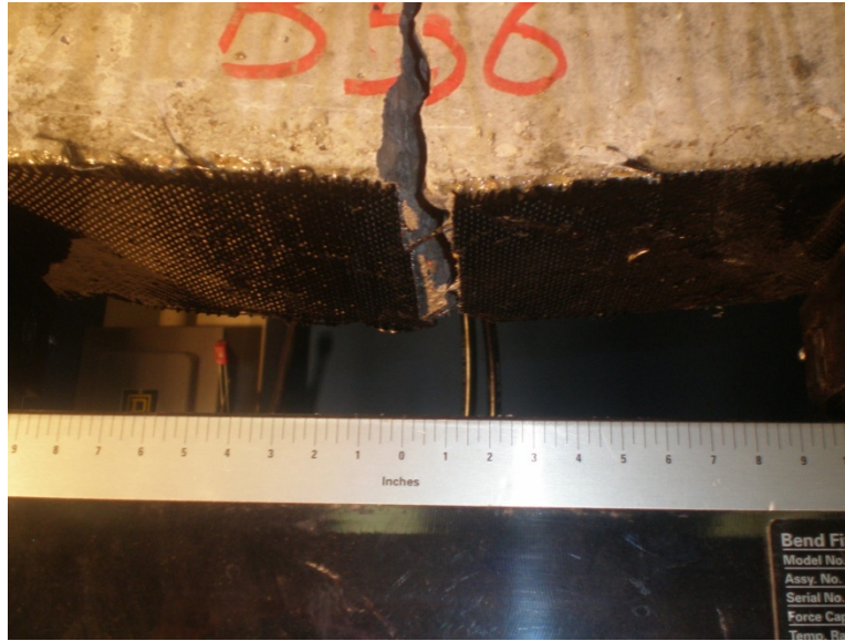
Figure 6.112: Typical mode of failure “FRP rupture” for concrete beam specimens (B56) at 100°C and 100 cycles
