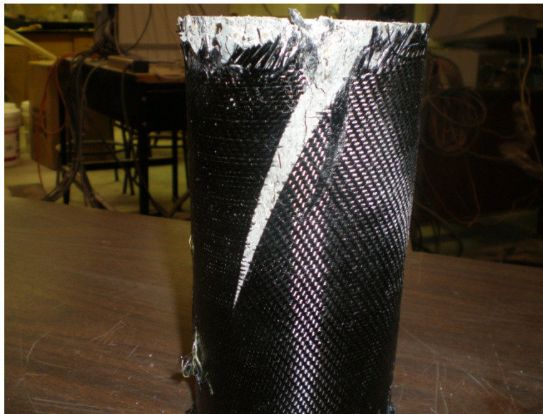
Figure 6.66: FRP rupture of concrete cylindrical specimen T
