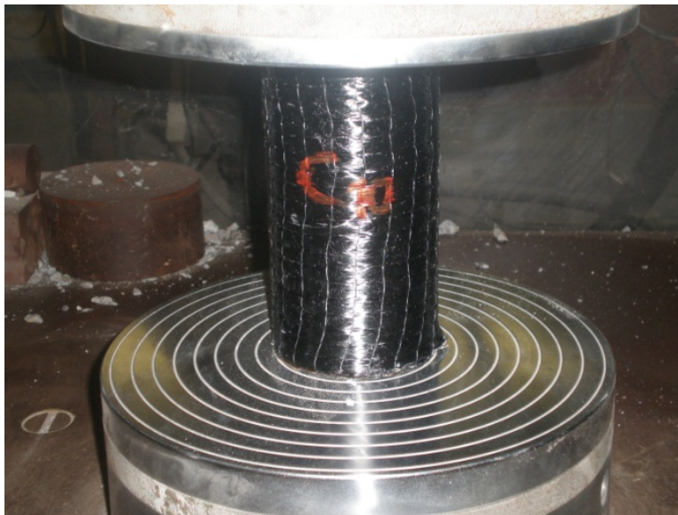
Figure 6.106: Compression strength test for column specimen strengthened by Fyfe CFRP and Sika epoxy
