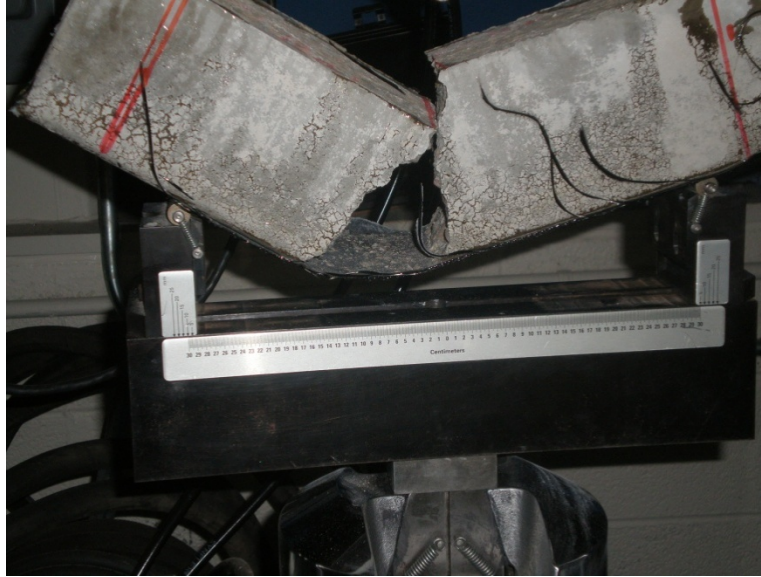
a) Concrete flexural crack, beam B1
