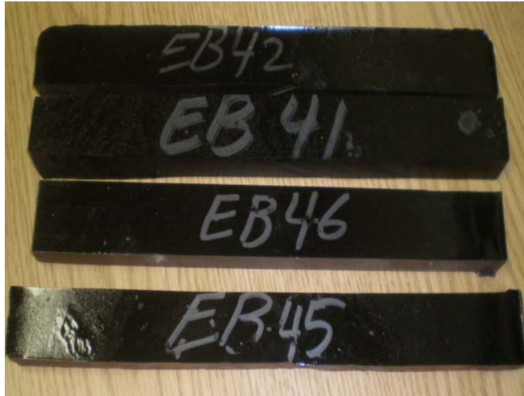
Figure 6.46: Color change to black after exposed to temperature of 180°C
