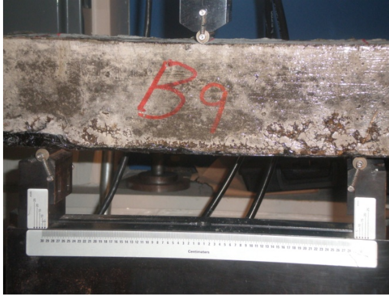
Figure 6.92: Beam specimens B9 strengthened by Fyfe CFRP and Sika epoxy
