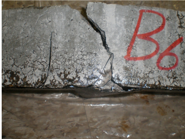
a) Concrete crushing, beam B6
