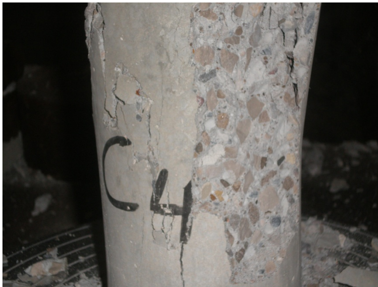
Figure 6.21: Compression failure of specimen C49 -100°C
