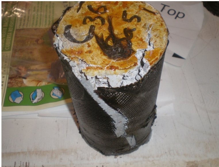
Figure 6.134: FRP rupture of C36-100°C, 625cycles
