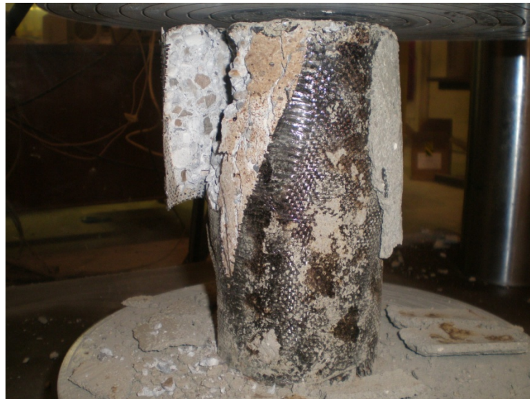
Figure 8.14: FRP rupture of protected column specimen
