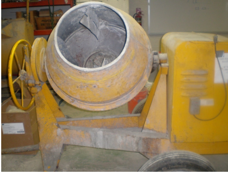
Figure 3.7: Heavy duty concrete mixer
