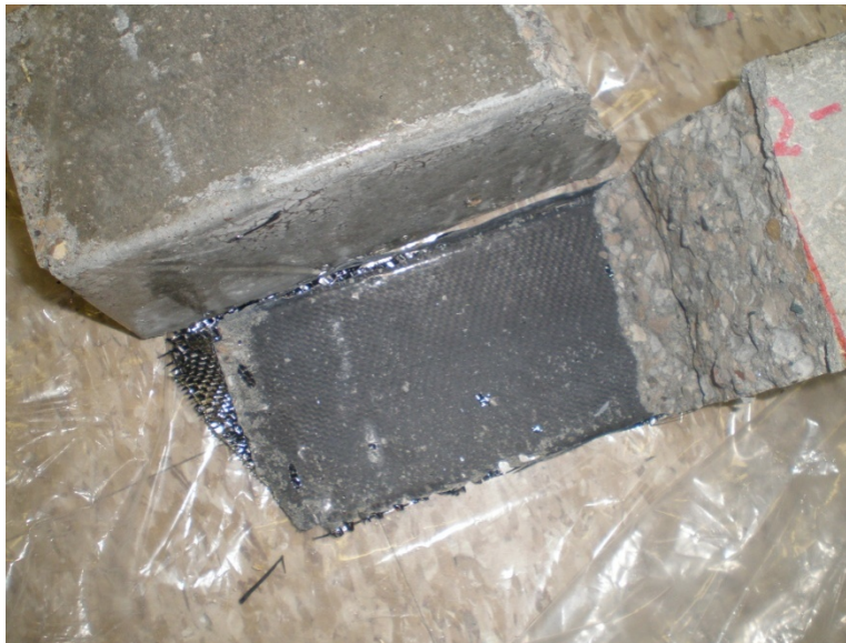
b) FRP delamination on concrete surface, beam B1
