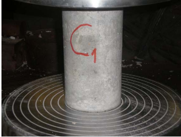
Figure 6.16: Compressive strength test C1 “control specimen”
