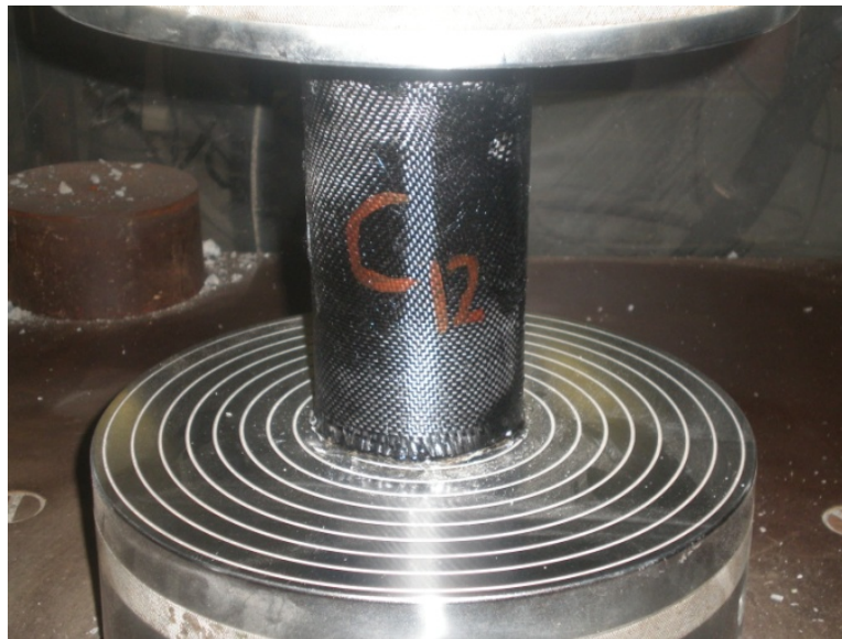
Figure 6.101: Compression strength test for column specimen strengthened by Sika CFRP and Fyfe epoxy
