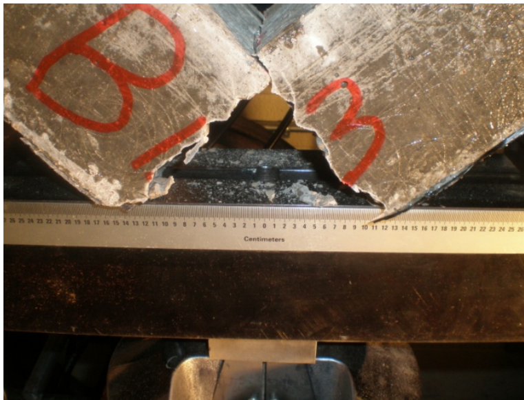
b) CFRP Rupture, B13
