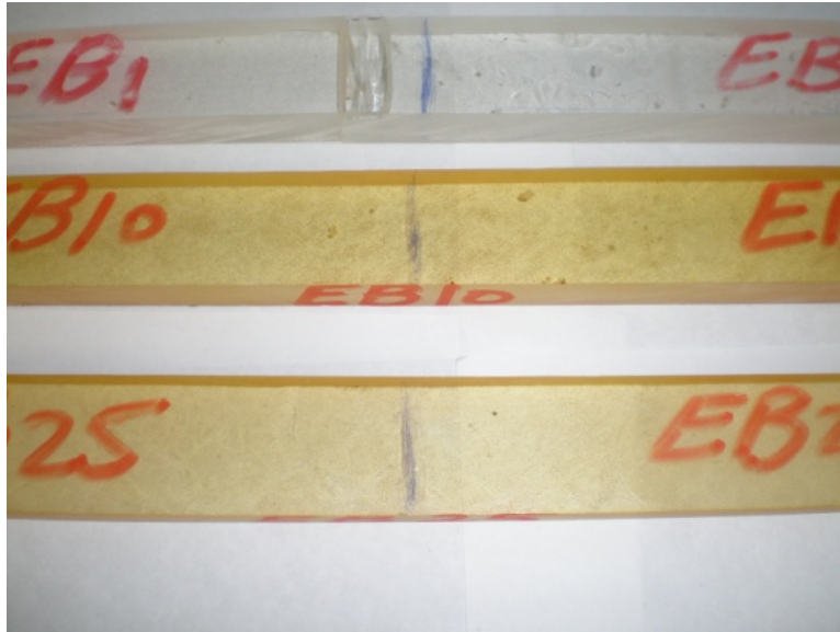
Figure 6.35: Changing of the specimens color at 40 cycles
