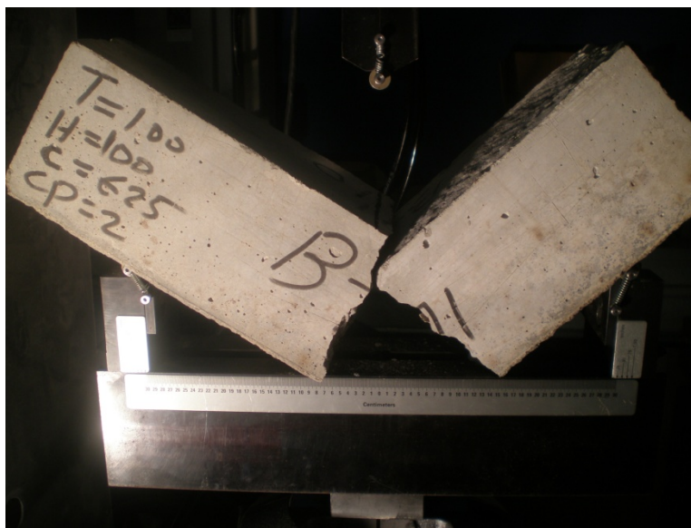
Figure 6.6: Flexural failure of concrete beam-100°C
