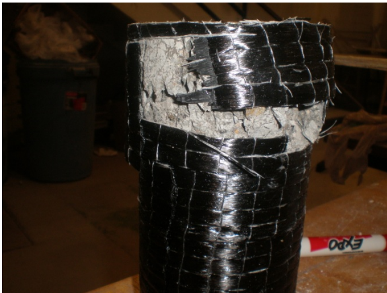
Figure 6.108: Hoop direction FRP rupture around the perimeter of the specimen, C10
