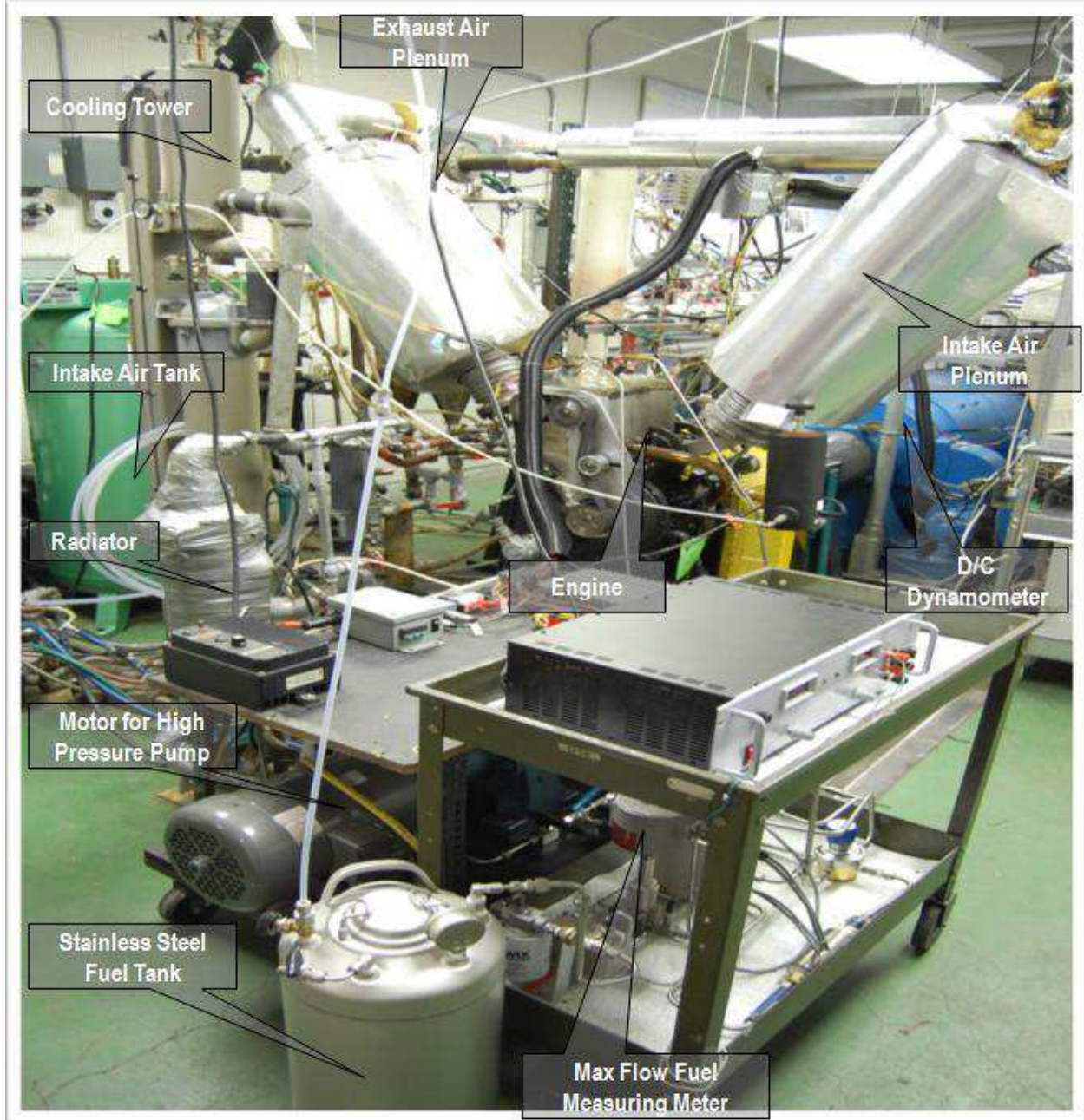
Figure 3.1: HSDI engine test cell
