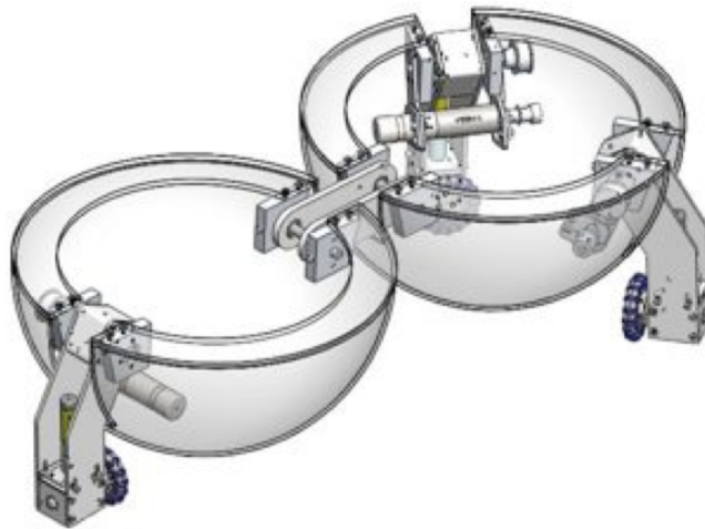
Figure 1.11: Image of spherical robot after reconfiguration [21].
