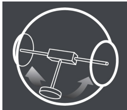
Figure 1.6: A commercialized pendulum-driven robot, Rotundus [13].
